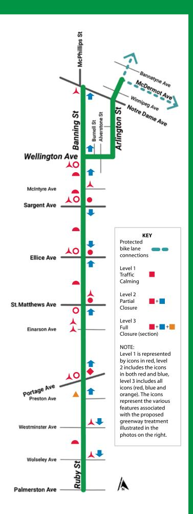
The following are proposed neighbourhood greenway treatments. Each level of treatment has the potential to calm traffic on the street by impacting traffic flow, and vehicle, pedestrian and bicycle speed. Treatments selected will be determined in the final design stage, including public feedback. Opportunities are available to tailor treatment levels based on the unique conditions throughout the corridor.
