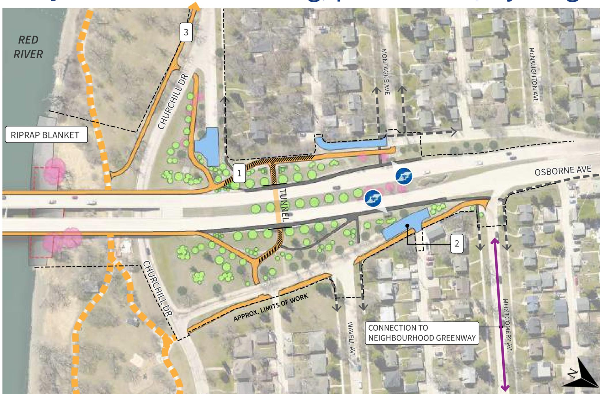
1. To provide an accessible 5% slope to the pedestrian tunnel, road closure on Churchill Drive is required
