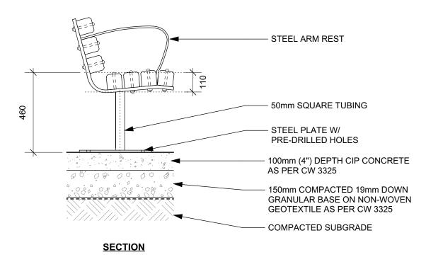
DIMENSIONS SHOWN ARE IN MILLIMETRES UNLESS OTHERWISE SPECIFIED
