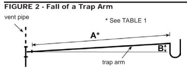
Developed length "A" must be at least twice the size of the trap arm. Fall "B" must not be greater than the size of the trap arm.
