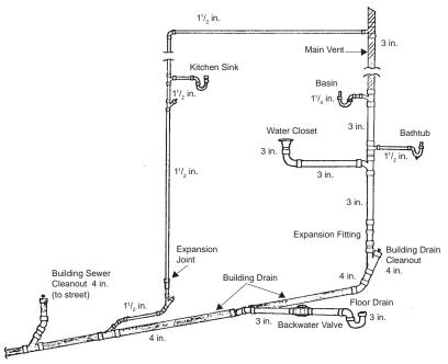
**Note:** Every building drain must be at least 100 mm. (4 in.) in size and must be terminated by a vent at least 75 mm (3 in.) in size.
