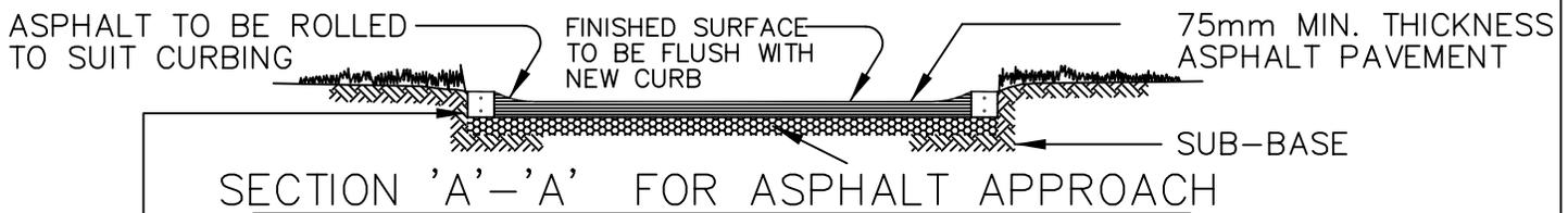
65mm x 140mm PRECAST OR 100mm x 200mm CAST-IN-PLACE CURB WITH TWO 15M DEFORMED BARS.
