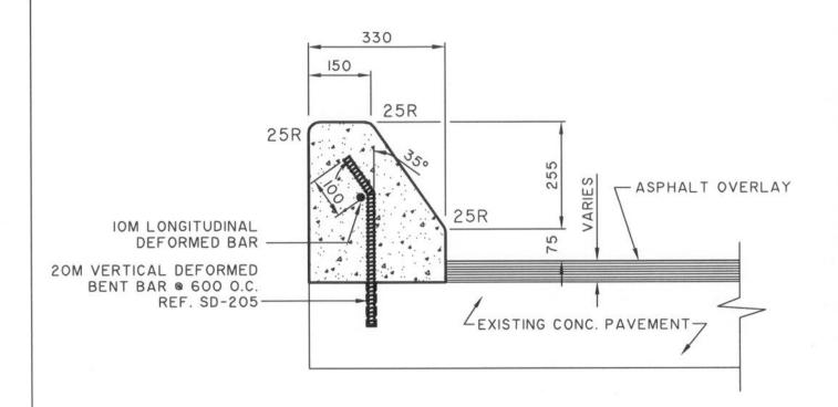
NOTE: TRANSVERSE SAW CUT EVERY 6000 OR AT PAVEMENT JOINTS.
