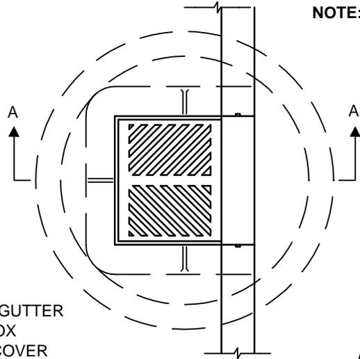
**NOTE:** EACH CATCH BASIN TO HAVE SEPARATE CONNECTION TO SEWER OR MANHOLE
