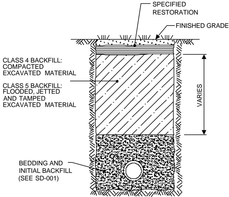
**CLASS 4 AND CLASS 5 BACKFILL**
