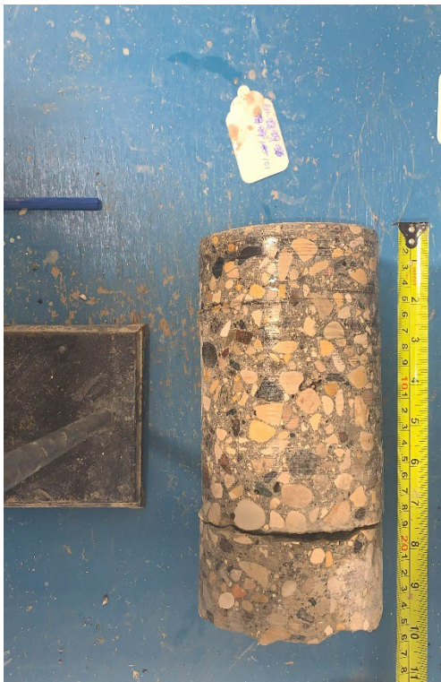
Figure 9 – Core Sample No. 101 – SB Curb Lane
