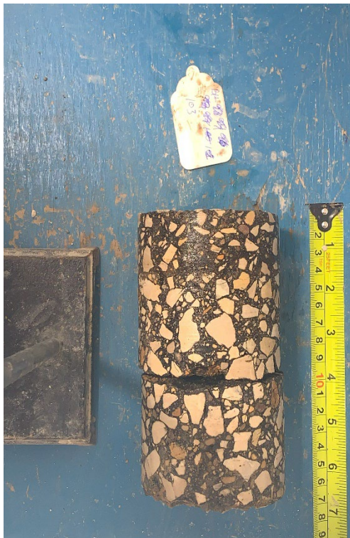
Figure 11 – Core Sample No. 103 – SB Curb Lane
