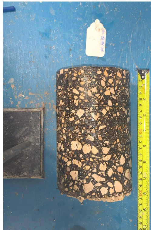
Figure 4 – Core Sample No. 96 – SB Curb Lane
