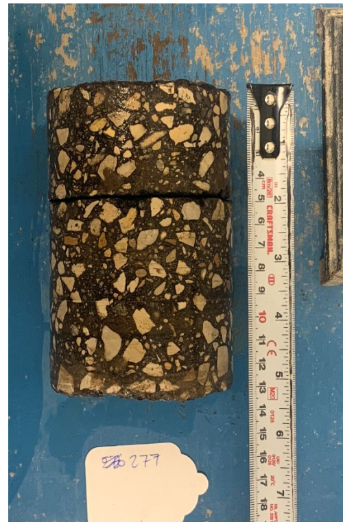
Figure 14 – Core Sample No. 277 – SB Shoulder
