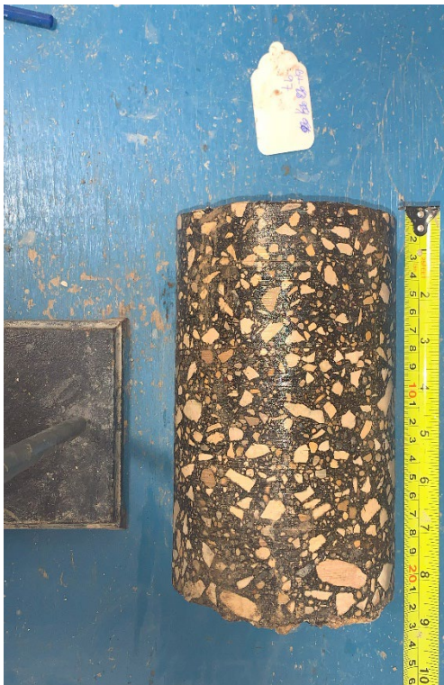
Figure 5 – Core Sample No. 97 – SB Curb Lane
