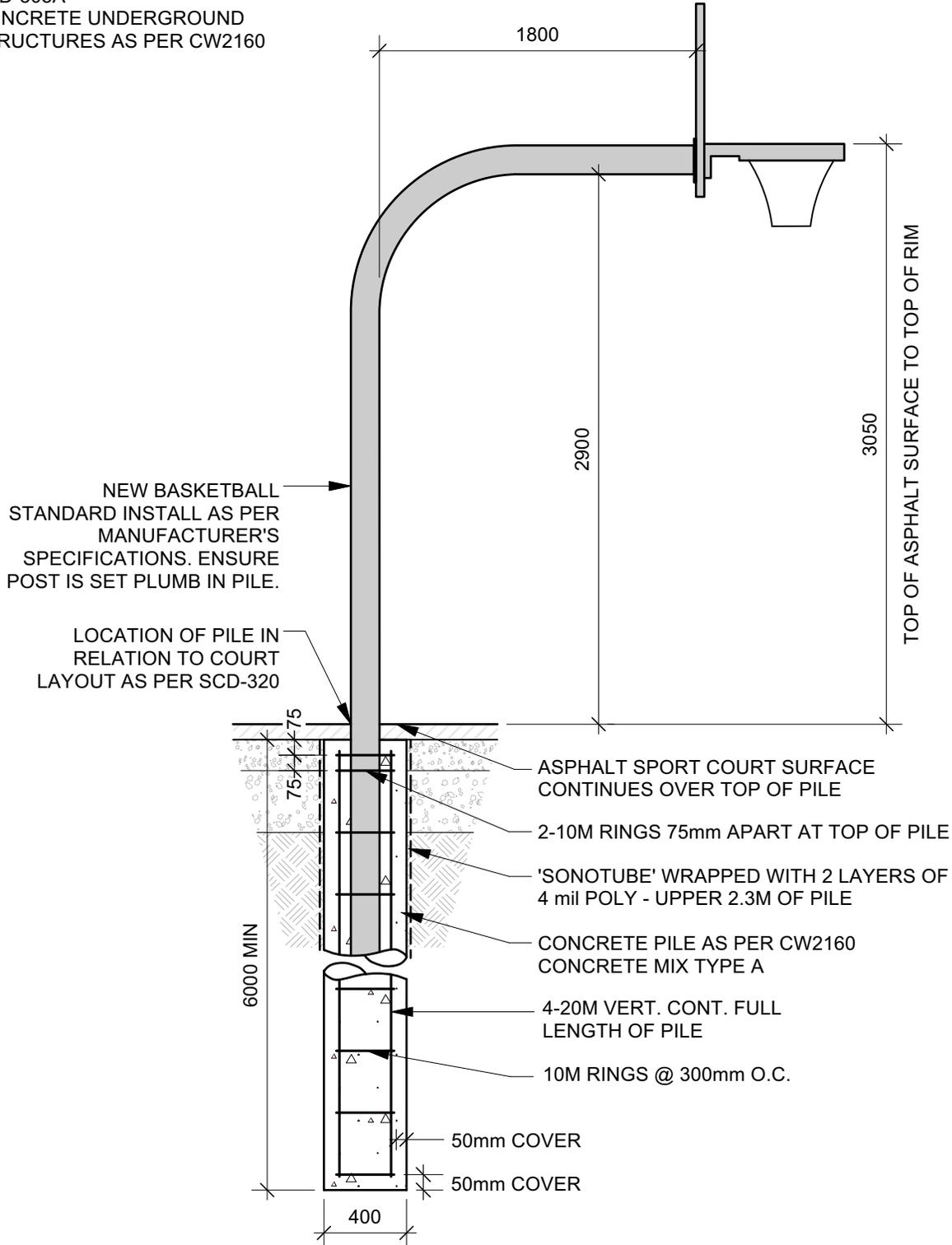
DIMENSIONS SHOWN ARE IN MILLIMETRES UNLESS OTHERWISE SPECIFIED
