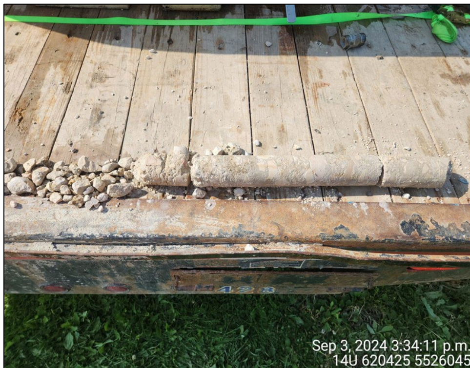
Photo 07: Core recovered from the limestone bedrock at TH24-03B.
