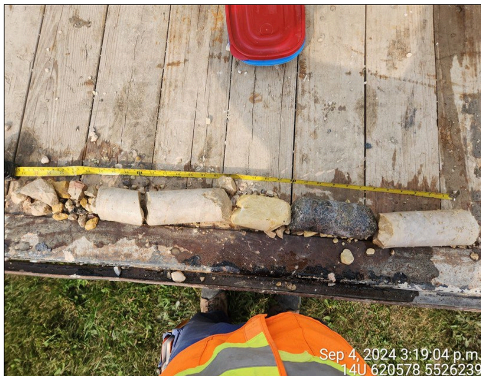
Photo 09: Core recovered from the sandy silt till at TH24-01B.
