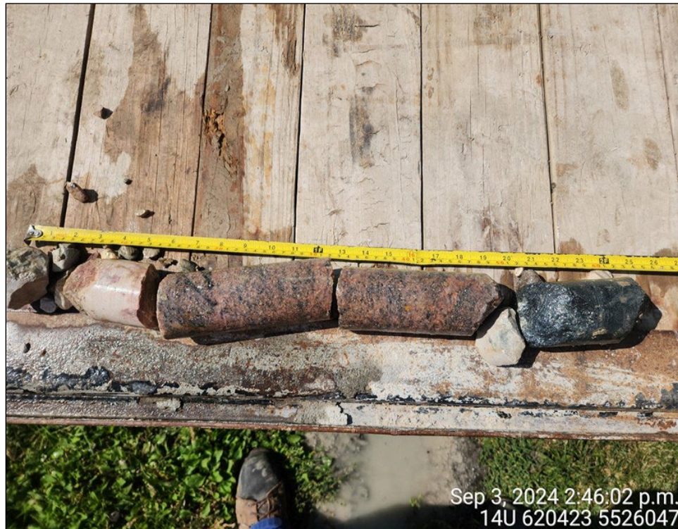
Photo 06: Core recovered from the sandy silt till at TH24-03B.
