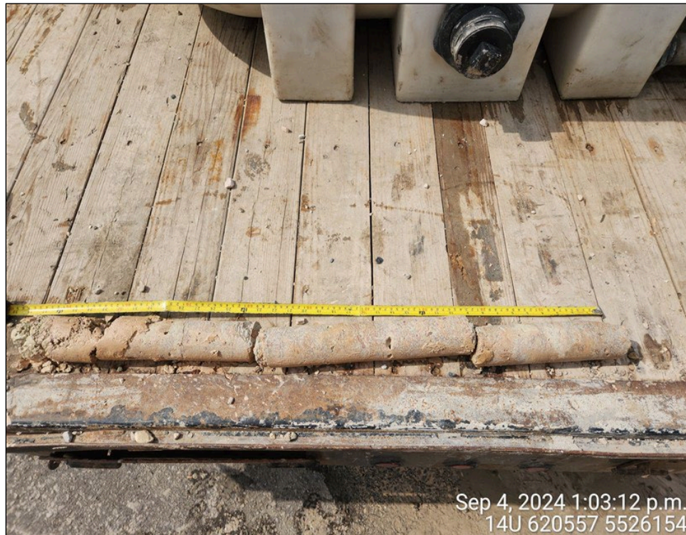
Photo 08: Core recovered from the limestone bedrock at TH24-02B.
