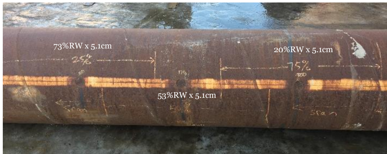
Figure 25. Calibration pipe with 73% RW, 53% RW, and 20% RW 5.1cm diameter flat bottom defects.
