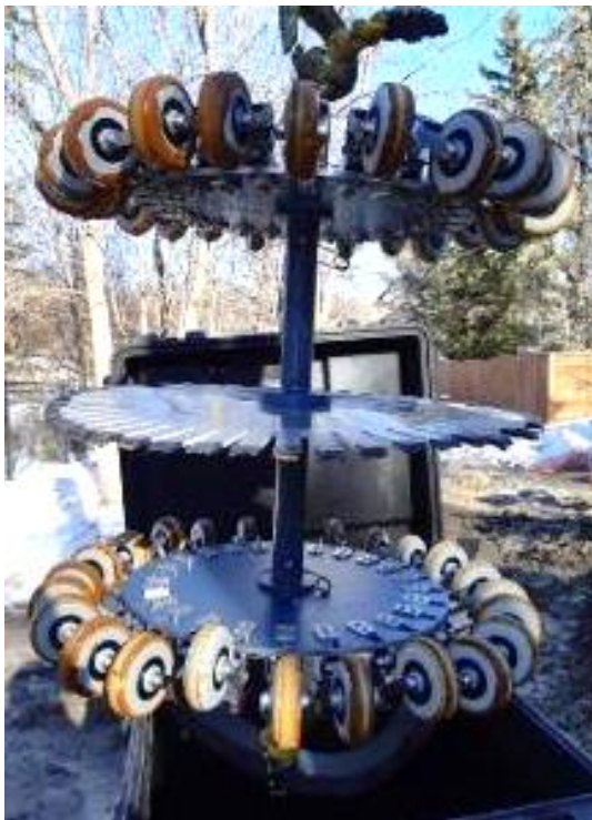
Figure 5. PICA's custom gauge tool assembly shown after being pulled through the Charleswood-Assiniboia Feeder Main
