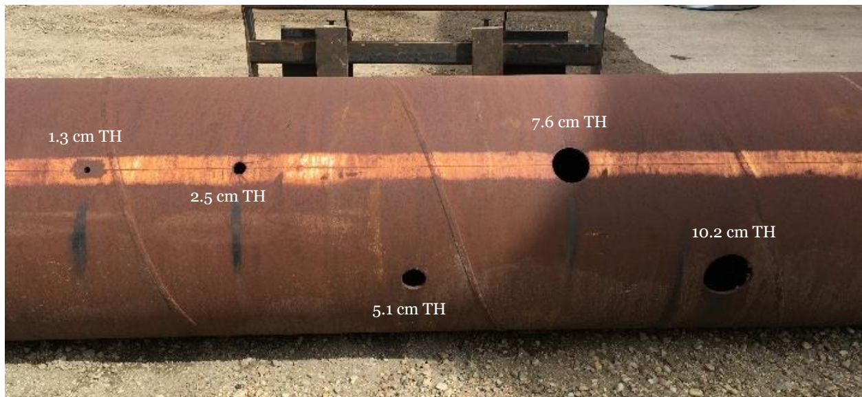
Figure 27. Through holes machined into the 24in calibration pipe. Defects measured 1.3 cm, 2.5 cm, 5.1 cm, 7.6 cm, and 10.2 cm (0.5in, 1.0in, 2.0in, 3.0in, and 4.0in) in diameter.
