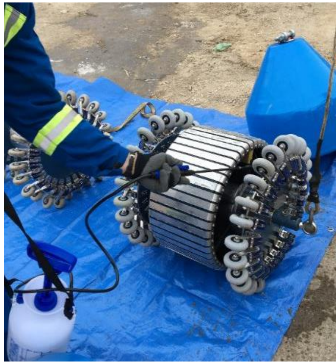
Figure 6. Disinfecting the Chimera assembly using a 200 mg/L free chlorine solution
