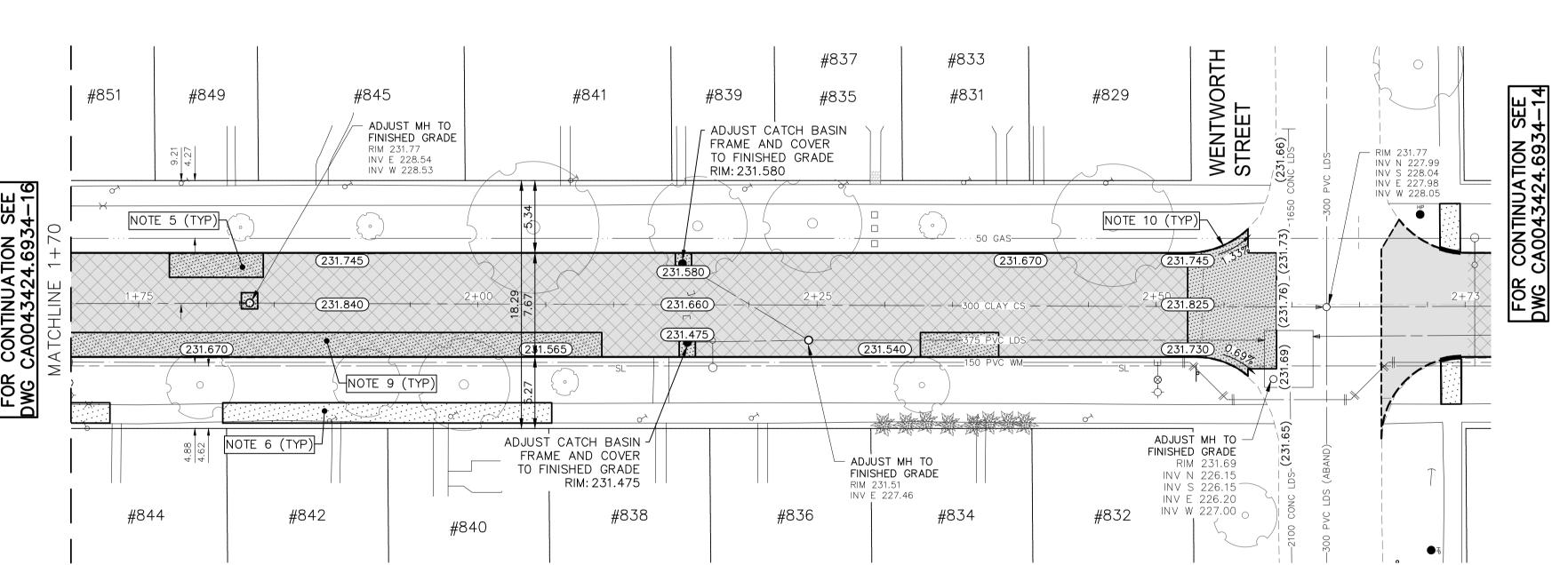
18.29 7.67 1.50 3.51 EX SWLK BOULEVARD BOULEVARD EX SWLK VARIES VARIES 2.0% 2.0% EXISTING BARRIER -70-90 mm ASPHALT PAVEMENT OVERLAY - EXISTING SIDEWALK TO BE CURB TO BE RENEWED TEXISTING 150mm CONCRETE PAVEMENT PARTIALLY RENEWED AS PER (DOWELLED, 100mm REVEAL) SD-228A AND AS DIRECTED BY AS PER SD-205 (TYP.) TYPICAL CROSS-SECTION CONTRACT ADMINISTRATOR (TYP.)
