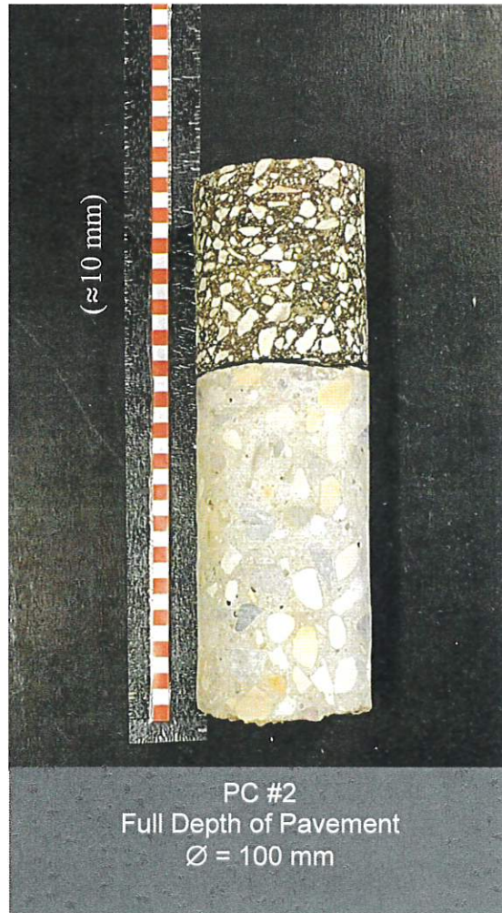
Photograph 2: Specimen from Bishop Grandin Boulevard, Eastbound Acceleration Lane
