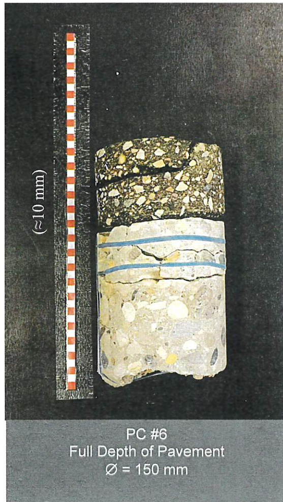
Photograph 6: Specimen from Bishop Grandin Boulevard, Westbound Lane Longitudinal Joint between Lanes
