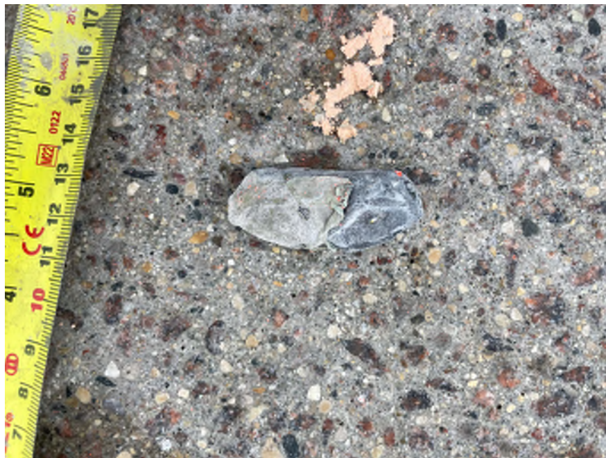
Photo 6 - Deck core D22, epoxy coated rebar condition, coated has failed and is debonding
