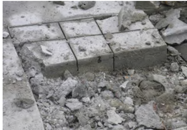
Photo 2.5 – Test Patch with Shallow Delamination
