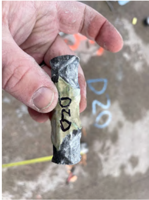
Photo 5 - Deck core D20, epoxy coated rebar condition, coated has failed and is debonding
