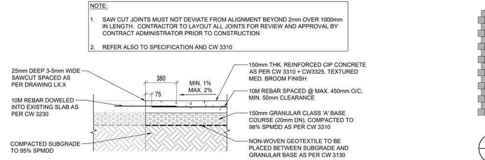
**2 REINFORCED PIP CONCRETE PAVING**
