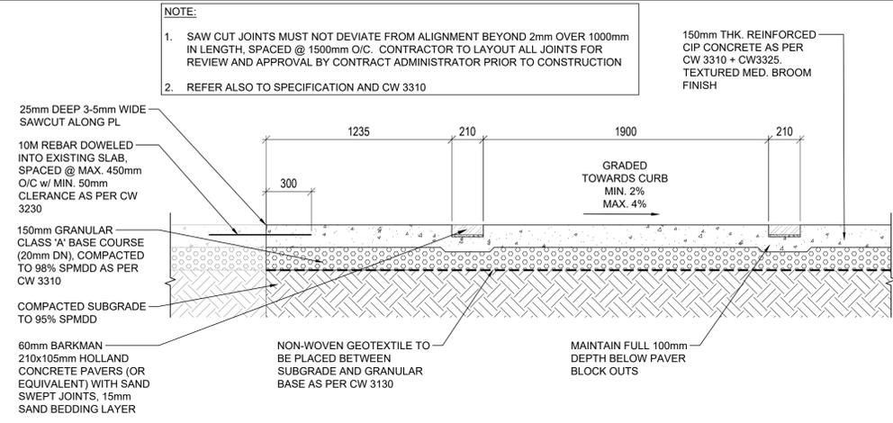
**1 R.O.W. CONCRETE PAVING w/ BLOCK OUTS**
