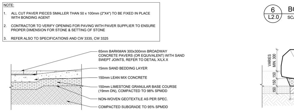
**4 PIP CONCRETE TO UNIT PAVEMENT TRANSITION**
