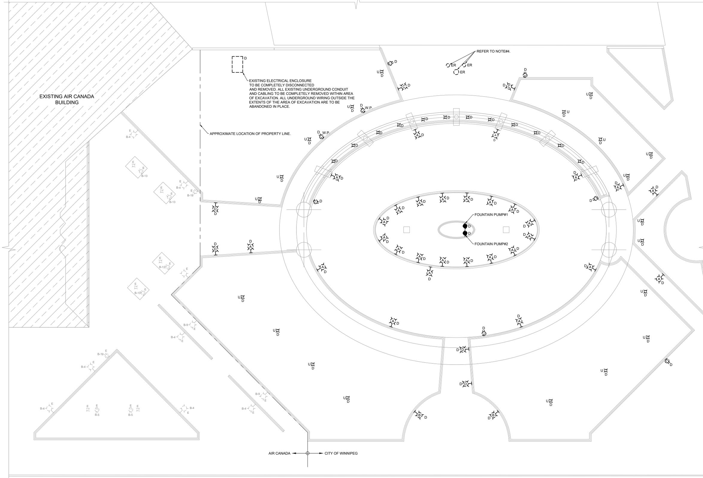
EXISTING ELECTRICAL ENCLOSURE TO BE COMPLETELY DISCONNECTED AND REMOVED. ALL EXISTING UNDERGROUND CONDUIT AND CABLEING TO BE COMPLETELY REMOVED WITHIN AREA OF EXCAVATION. ALL UNDERGROUND WIRING OUTSIDE THE EXTENTS OF THE AREA OF EXCAVATION ARE TO BE ABANDONED IN PLACE.
