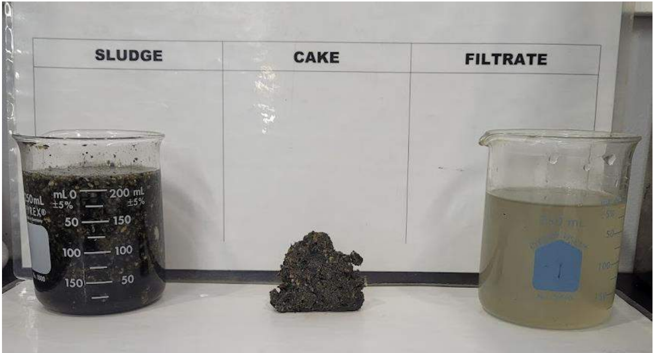
Raw sludge, cake & filtrate obtained during lab test
