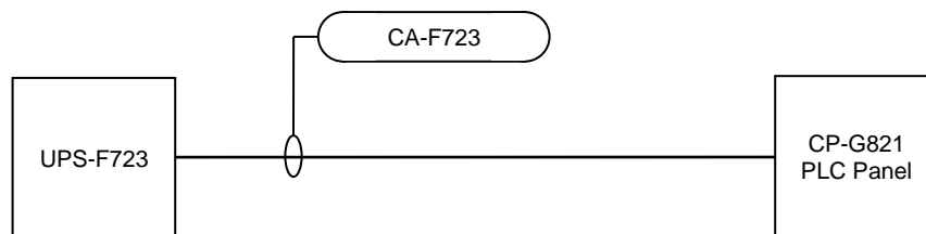
Figure 7-3: Instrument Cable Identification Example – Identified Equipment
