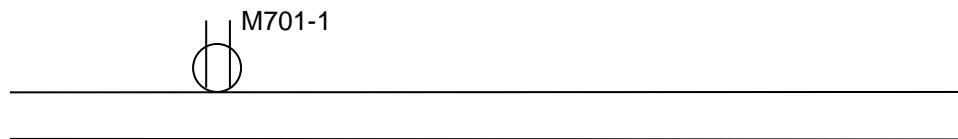
Figure 6-1 : Receptacle Identification on Plan Drawings
