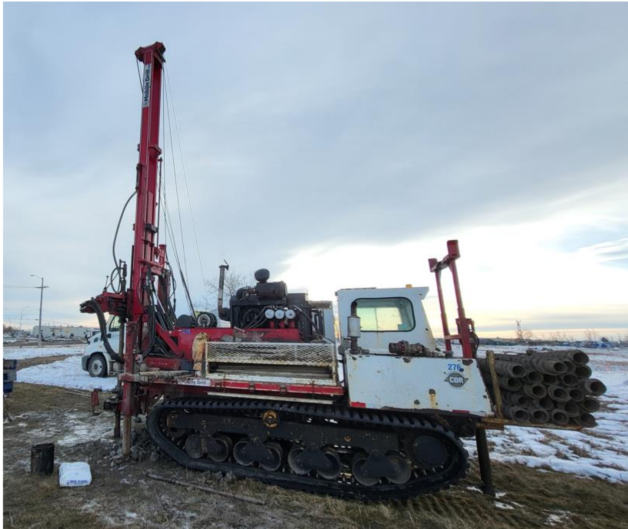
Figure 4 - Coring Conducted Onsite and Mobile B48 Drill Rig (TH24-09)
