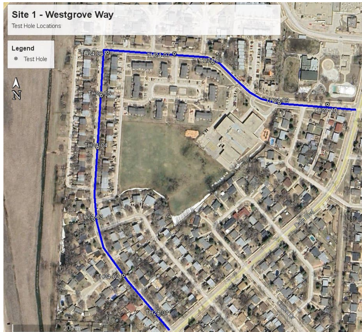
FIGURE 1: TEST HOLE LOCATIONS FOR WESTGROVE WAY
