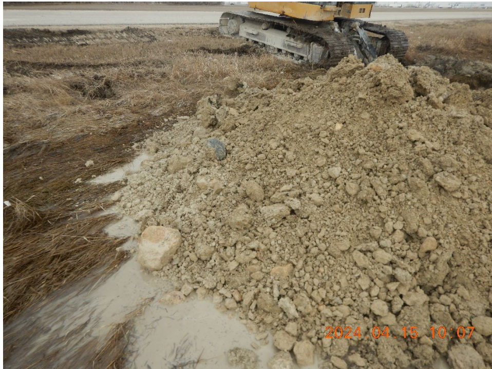
TP24-05 Photo 3: Cobbles and boulders in silt till
