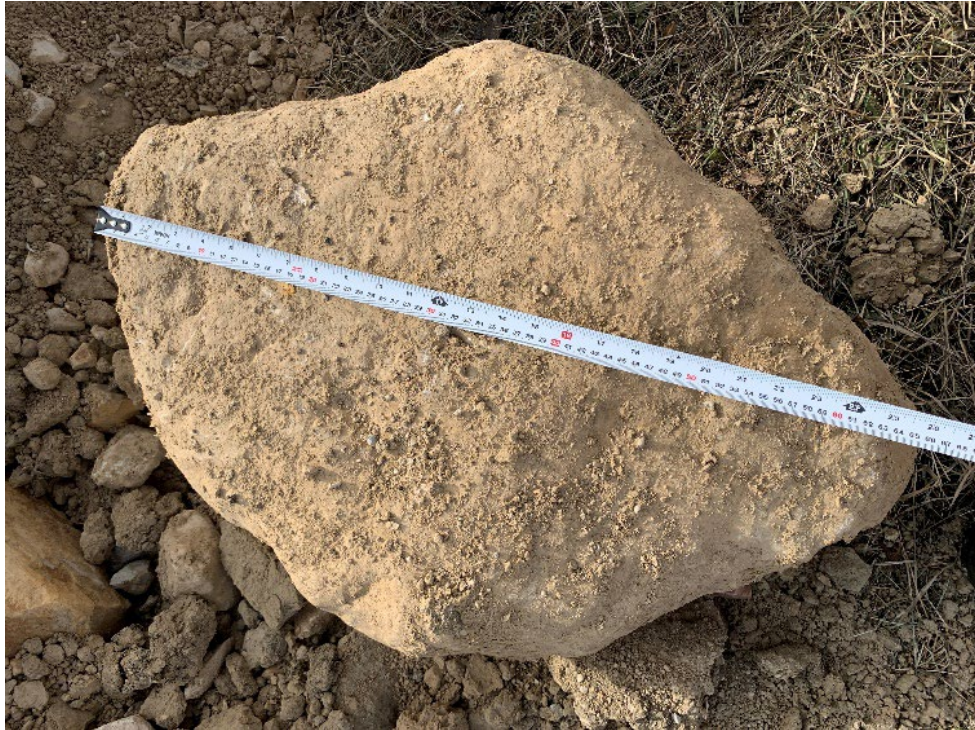
TP24-02 Photo 5: Boulder from silt till (24 inches)
