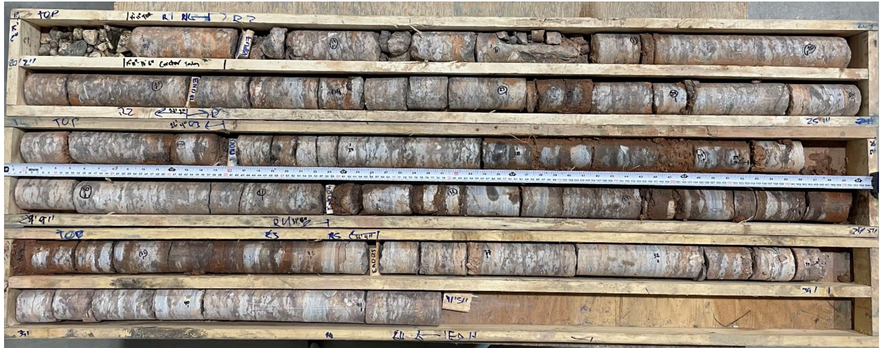
TH23-18 Photo 4: Bedrock core from 4.6 m to 12.4 m (15 ft – 5 in to 41 ft – 5 in)
