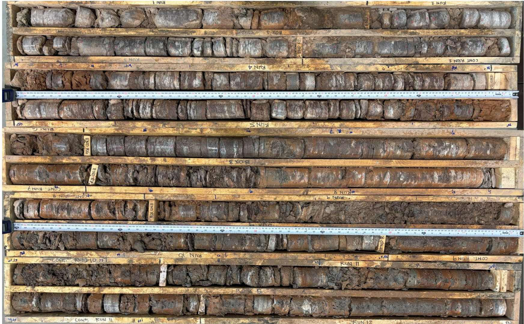
TH24-02 Photo 1: Bedrock core from 4.9 m to 21.5 m (16 ft to 70 ft – 6 in)
