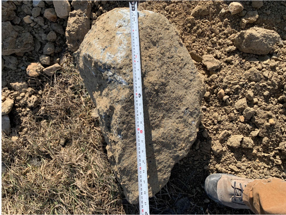
TP24-02 Photo 3: Boulder from silt till (22 inches)
