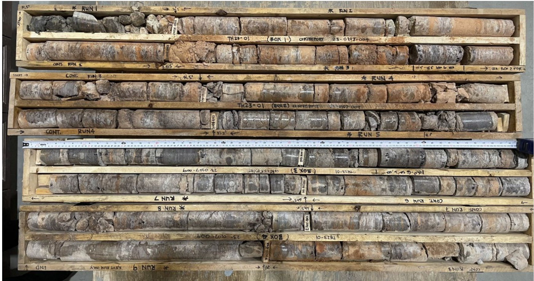
TH23-01 Photo 7: Bedrock Core, 9.45 m to 22.2 m (31.5 ft to 74 ft)
