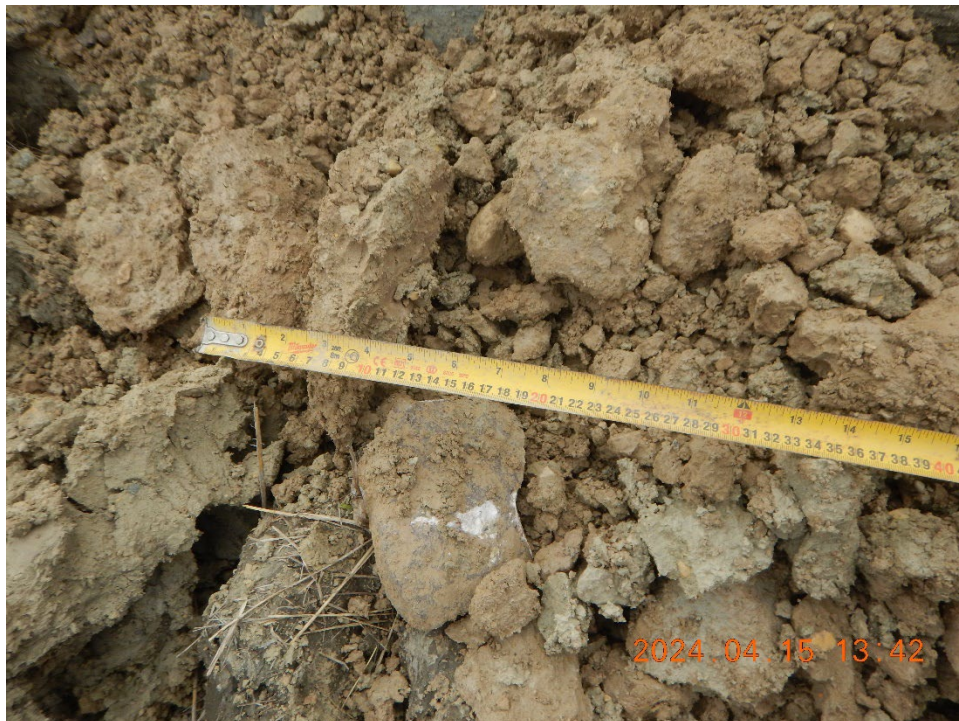
TP24-03 Photo 2: Cobbles encountered in silt till
