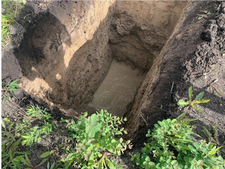
TP24-06 (North) Photo 1: Groundwater encountered at 3.6 m
