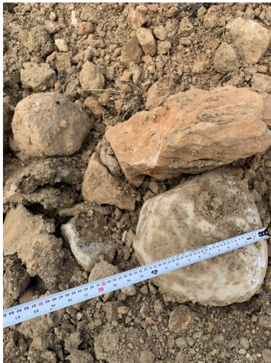
TP24-01 Photo 4: Boulders from Silt Till
