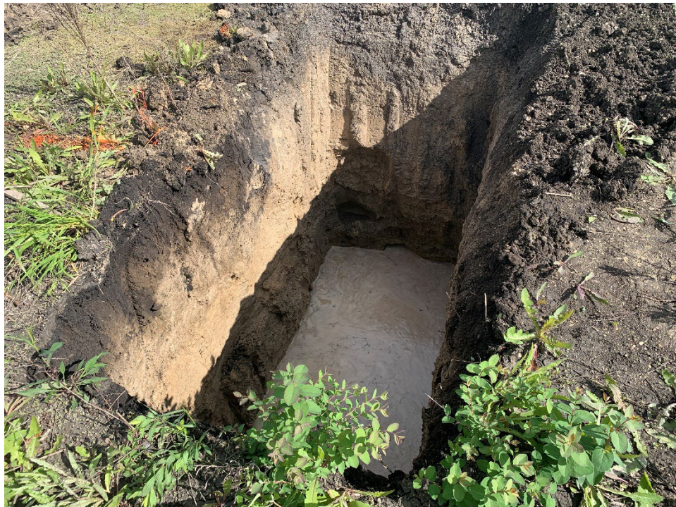
TP24-06 (North) Photo 2: Static groundwater at 2.1 m depth below ground surface upon completion of test pit excavation
