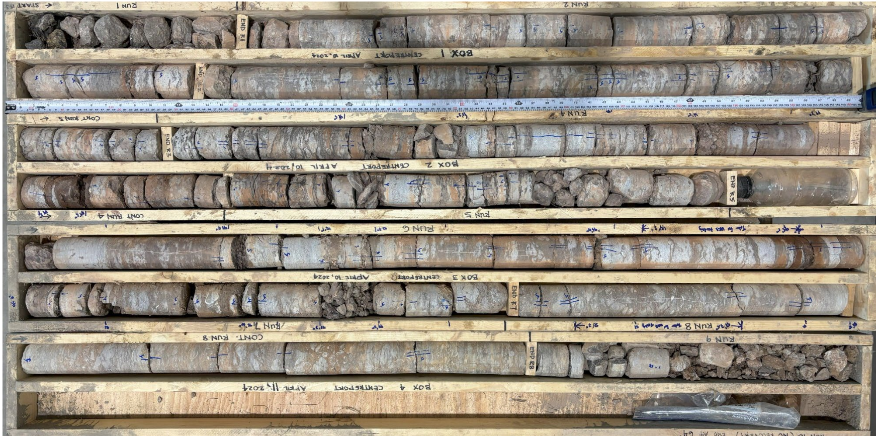
TH24-01 Photo 1: Bedrock core from 5.9 m to 19.5 m (19 ft – 6 in to 64 ft – 0 in)
