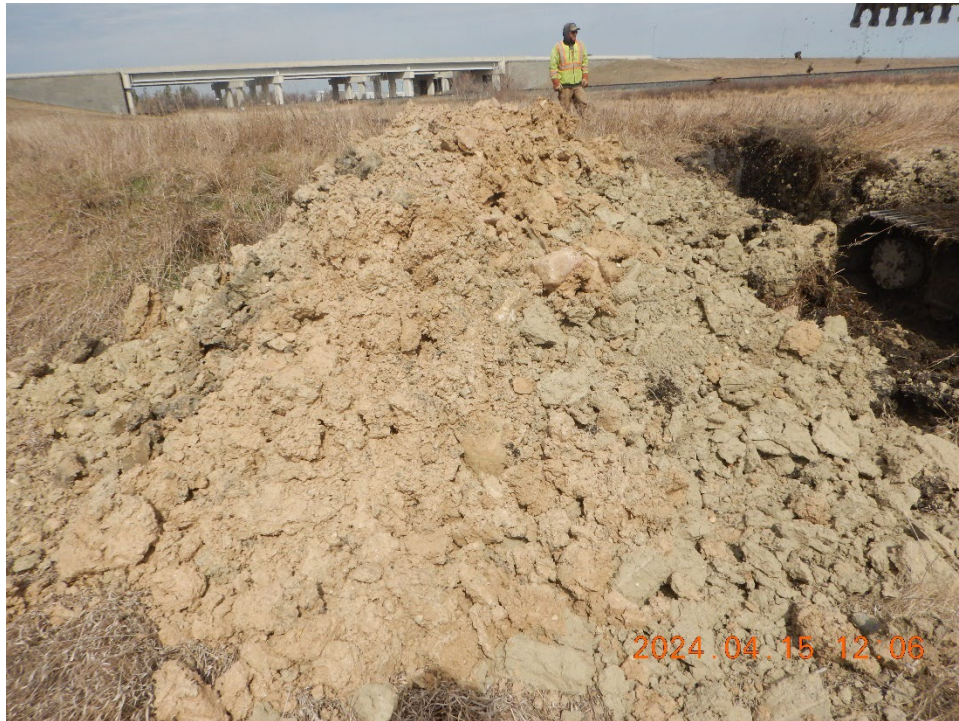
TP24-04 Photo 3: Cobbles and trace boulders in silt till
