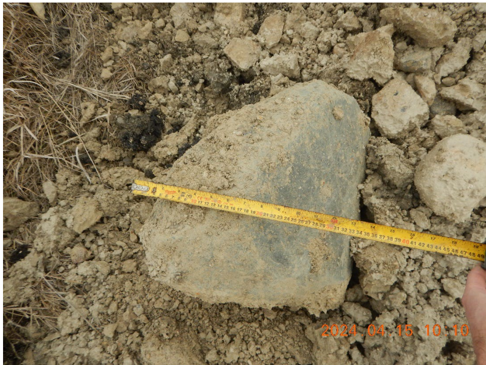
TP24-05 Photo 3: Igneous boulder in silt till
