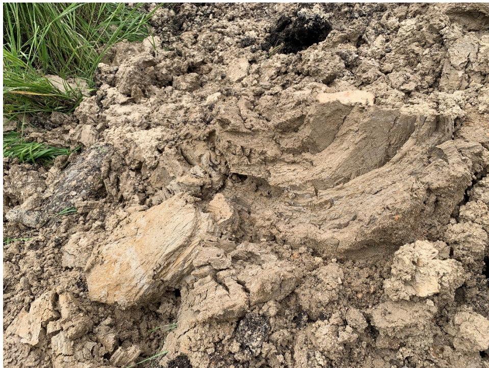
TP24-06 (North) Photo 4: Laminated sandy silt pocket encountered above silt till
