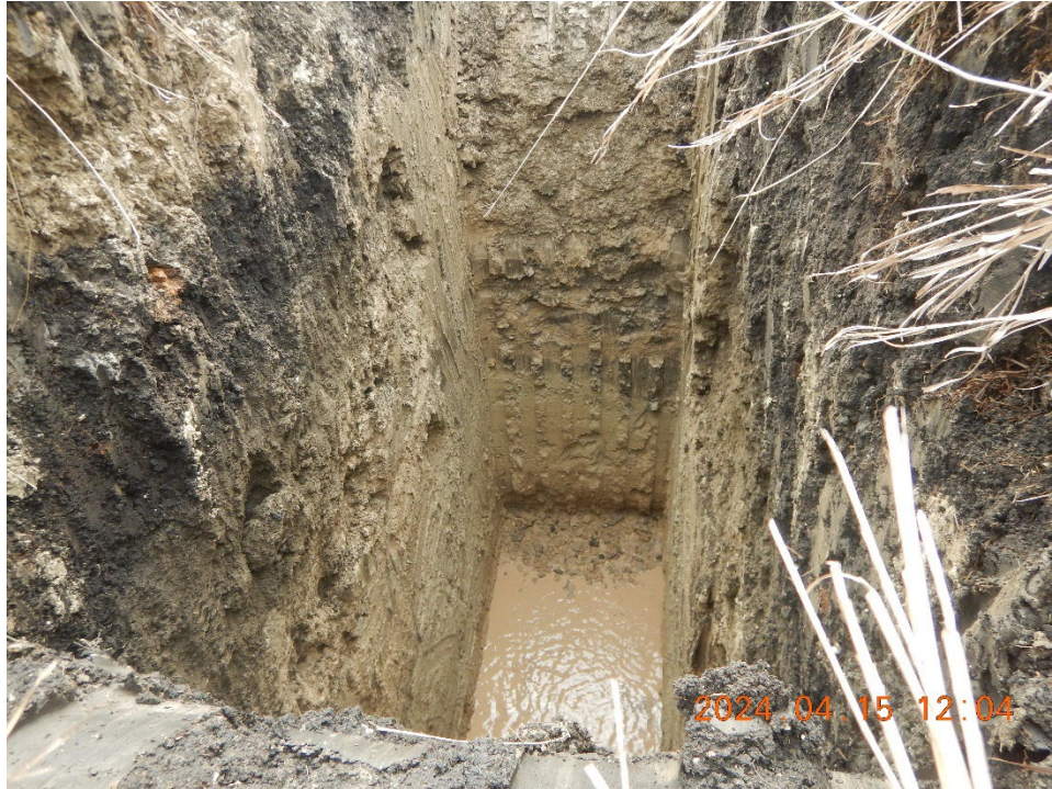
TP24-04 Photo 1: Top of bedrock encountered at 5.2 m
