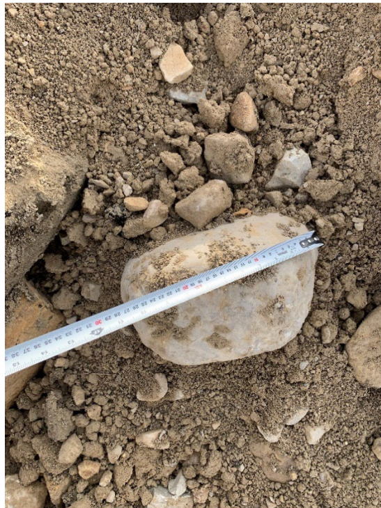
TP24-02 Photo 6: Igneous boulder in silt till
