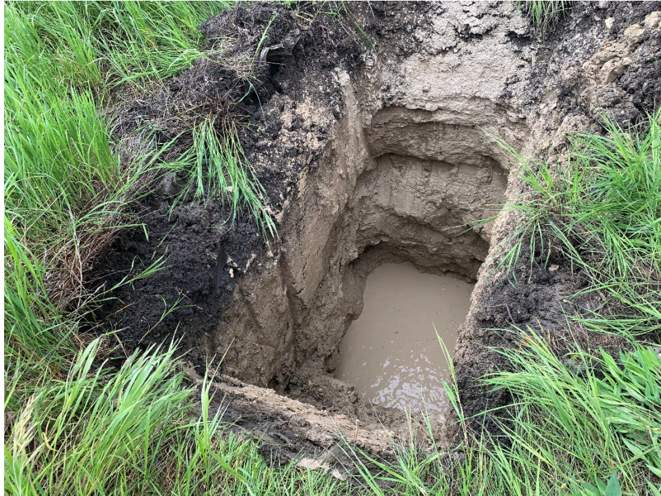
TP24-06 (South) Photo 1: Groundwater encountered at 3.6 m
