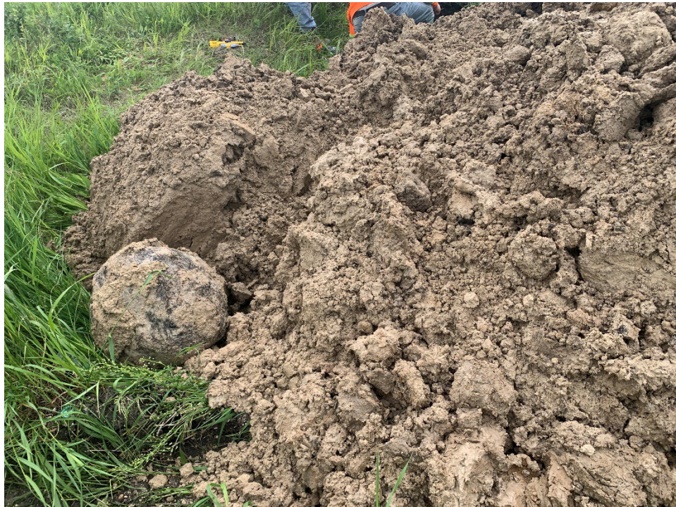
TP24-06 (South) Photo 2: Overview of silt till and boulder excavated from test pit
