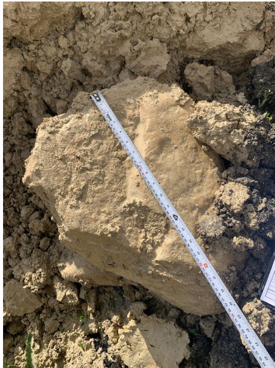
TP24-06 (North) Photo 4: Sedimentary boulder in silt till
