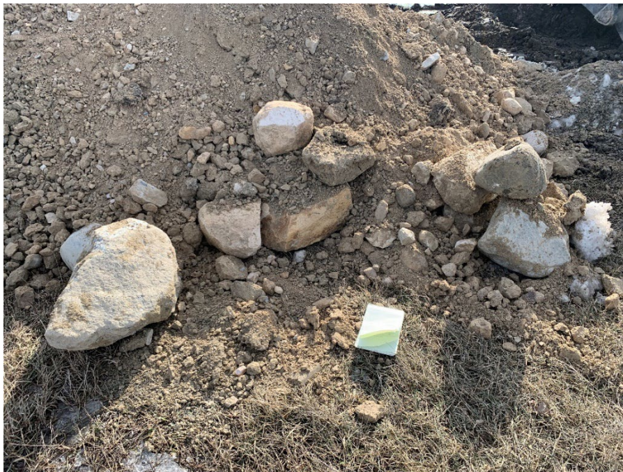
TP24-02 Photo 2: Cobbles and Boulders from silt till
