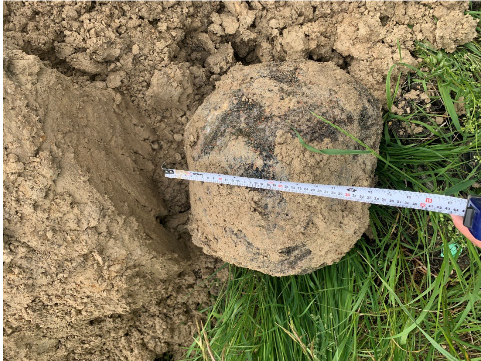
TP24-06 (North) Photo 3: Igneous boulder in silt till
