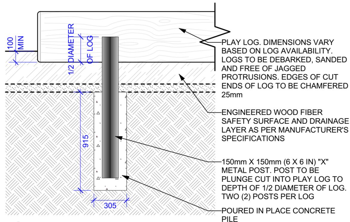
PLAY LOG. DIMENSIONS VARY BASED ON LOG AVAILABILITY. LOGS TO BE DEBARKED, SANDED AND FREE OF JAGGED PROTRUSIONS. EDGES OF CUT ENDS OF LOG TO BE CHAMFERED 25mm
