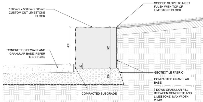
**1** LIMESTONE RETAINING WALL DETAIL
