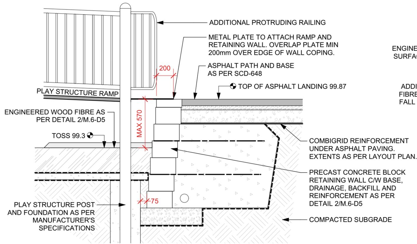
1 **RETAINING WALL AT RAMP**
