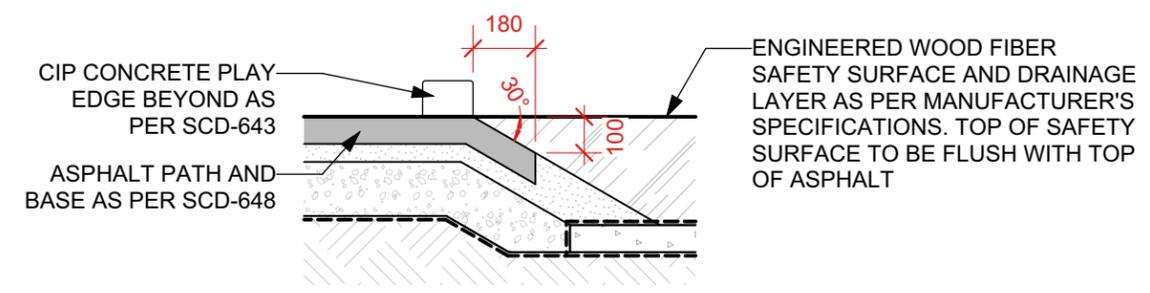
4 **ACCESSIBLE ROLLED ASPHALT ENTRY**
