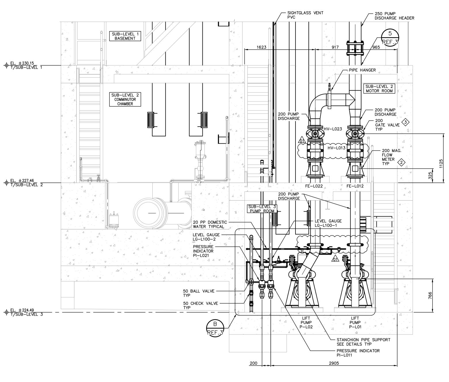
LIFT STATION SECTION LOOKING WEST SCALE: 1:25
