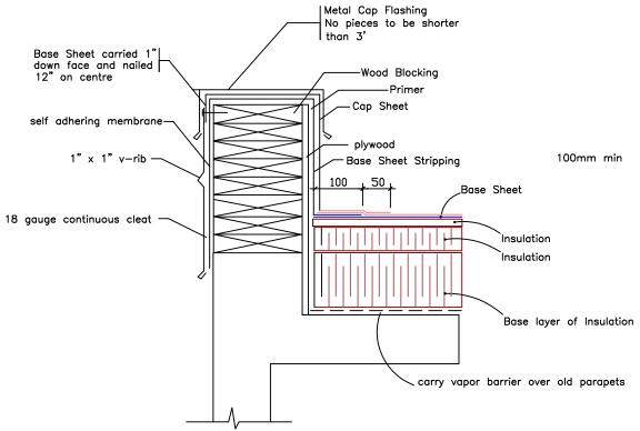
A continuous 18 gauge galvanized cleat is to be installed to insure outside face of flashing is firmly attached to outside face whenever outside face of flashing exceeds 3". No fasteners will be accepted on the outside face.
