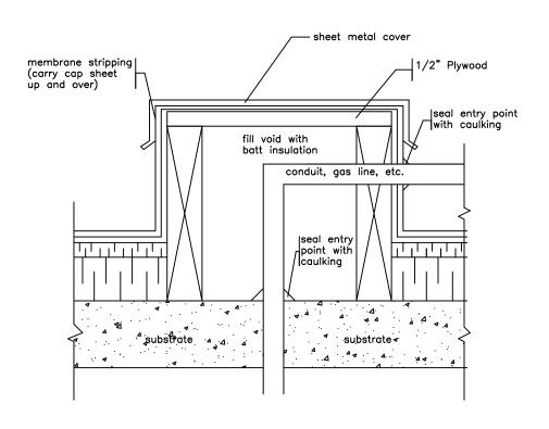
Note: vapour barrier is to be carried under curb curb height is to be minimum 12" above top of new roofing
