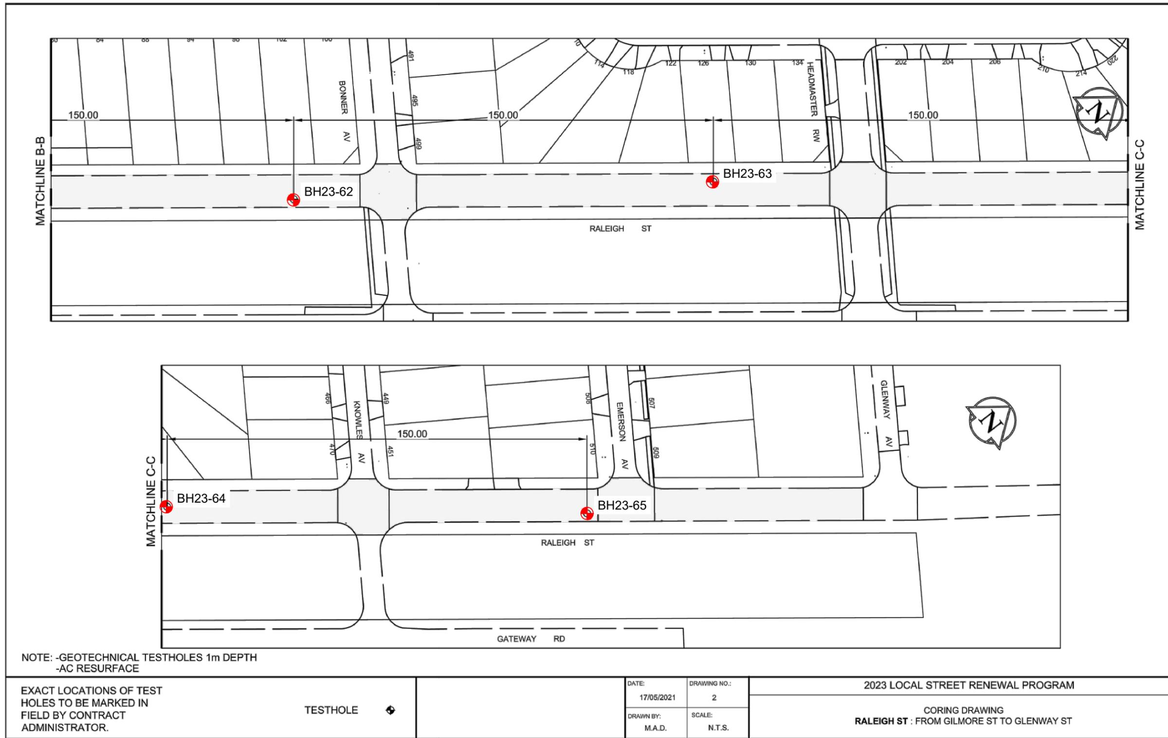
NOTE: -GEOTECHNICAL TESTHOLES 1m DEPTH
