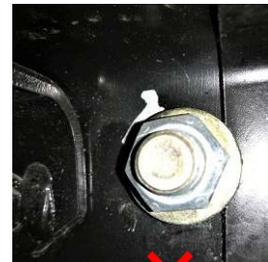
Bolt/nut assembly through chassis frame. If hole is where a transition occurs or on a curved surface in the frame the hole should not be used as a mounting location. However, if the hole location is to be used as a mounting location the following must be followed:
