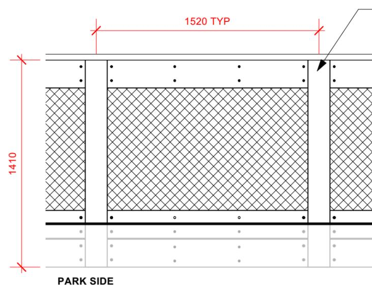
**1** **TIMBER FENCE ELEVATION**
