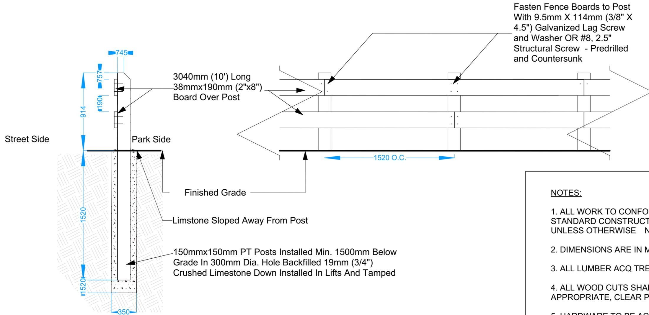
Fasten Fence Boards to Post With 9.5mm X 114mm (3/8" X 4.5") Galvanized Lag Screw and Washer OR #8, 2.5" Structural Screw - Predrilled and Countersunk
