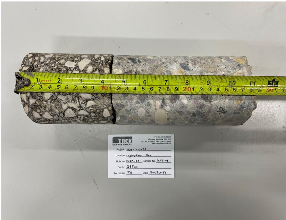
Photo 8: Pavement Core Sample PC-08
