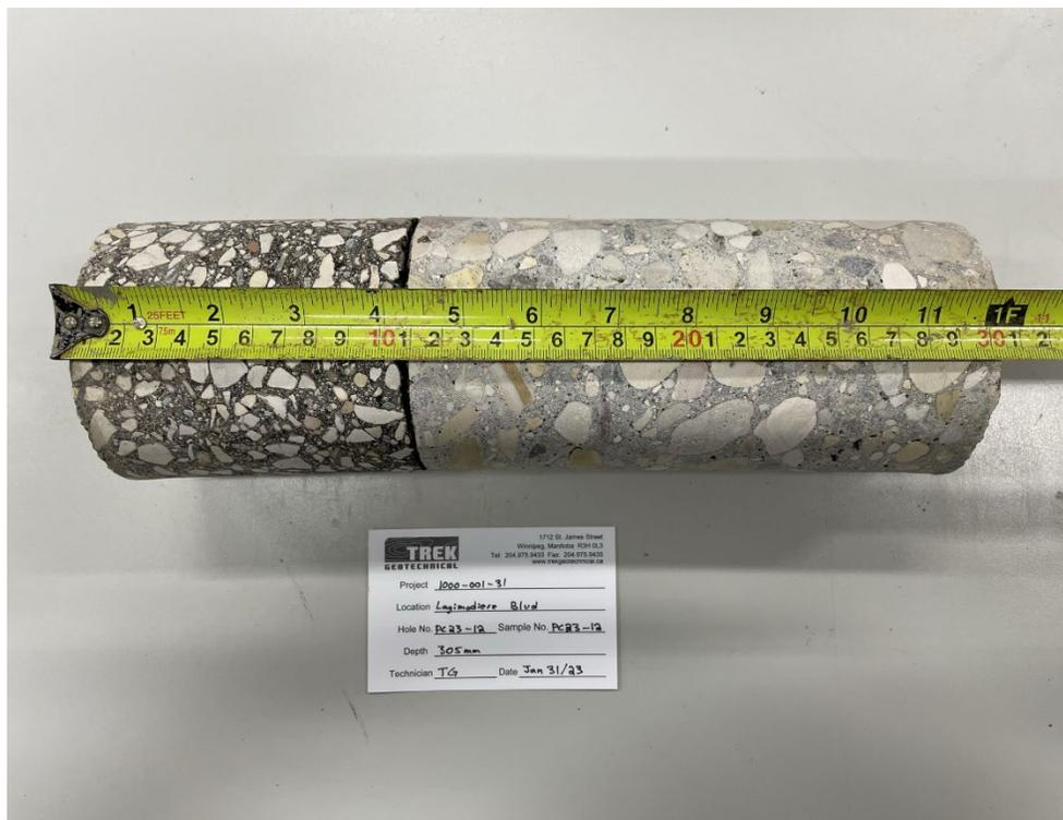
Photo 12: Pavement Core Sample PC-12
