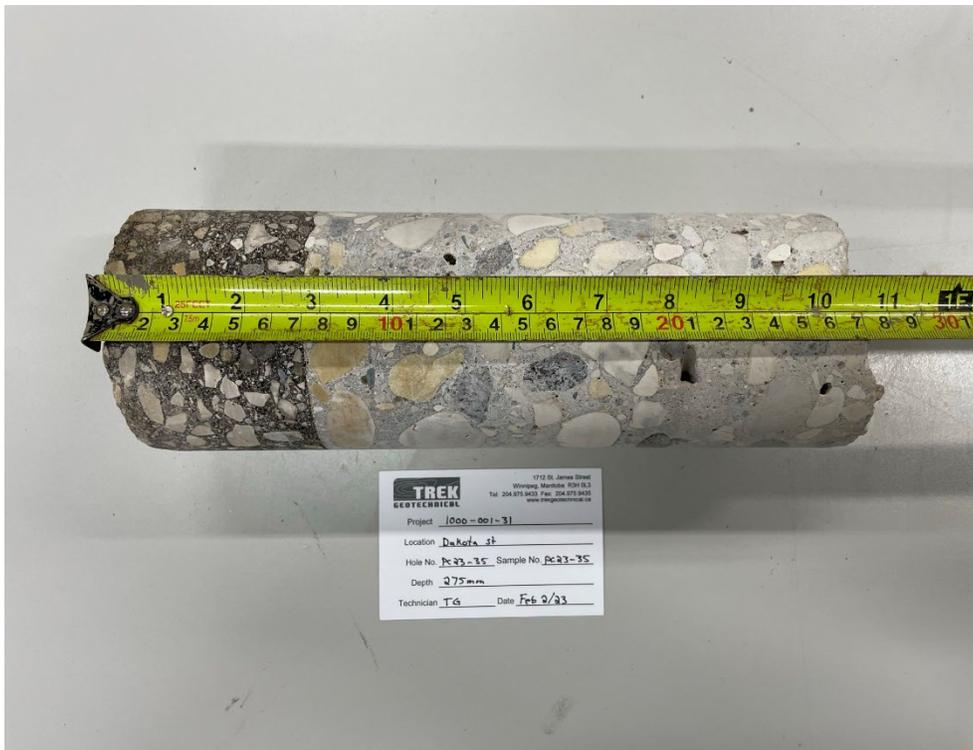
Photo 16: Pavement Core Sample PC-35
