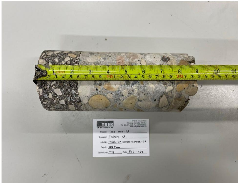
Photo 10: Pavement Core Sample PC-29
