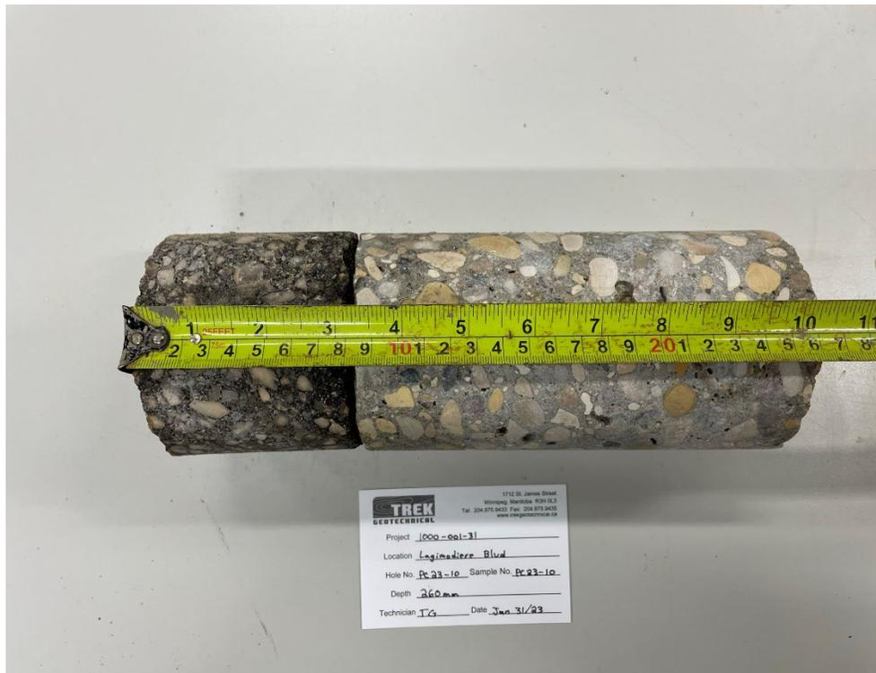
Photo 10: Pavement Core Sample PC-10
