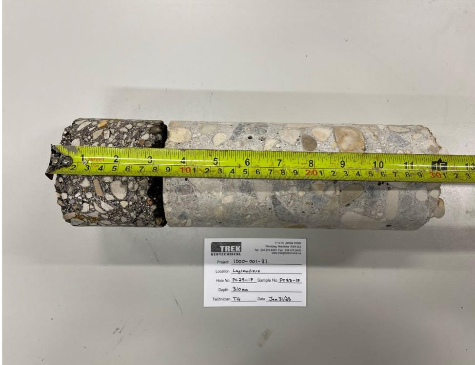
Photo 19: Pavement Core Sample PC-19
