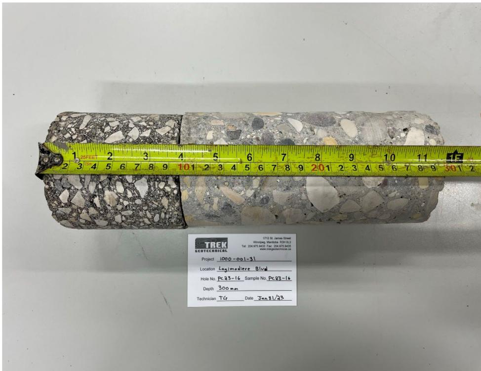
Photo 16: Pavement Core Sample PC-16
