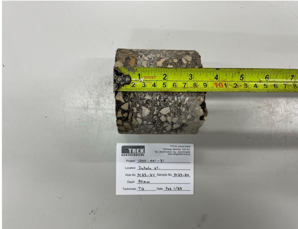
Photo 5: Pavement Core Sample PC-24
