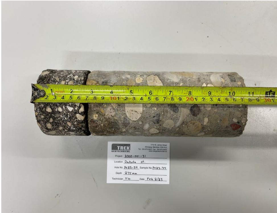
Photo 15: Pavement Core Sample PC-34
