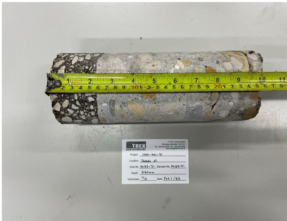
Photo 12: Pavement Core Sample PC-31
