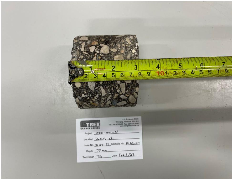
Photo 8: Pavement Core Sample PC-27
