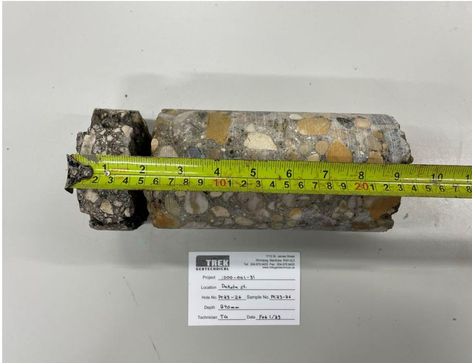
Photo 7: Pavement Core Sample PC-26
