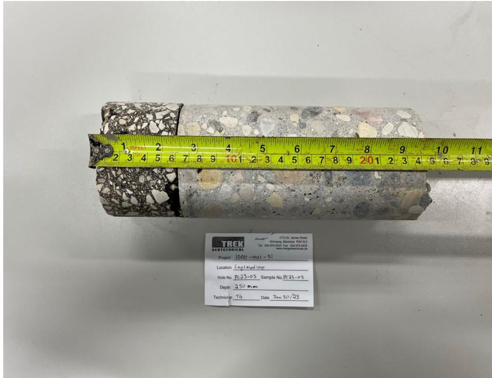
Photo 3: Pavement Core Sample PC-03
