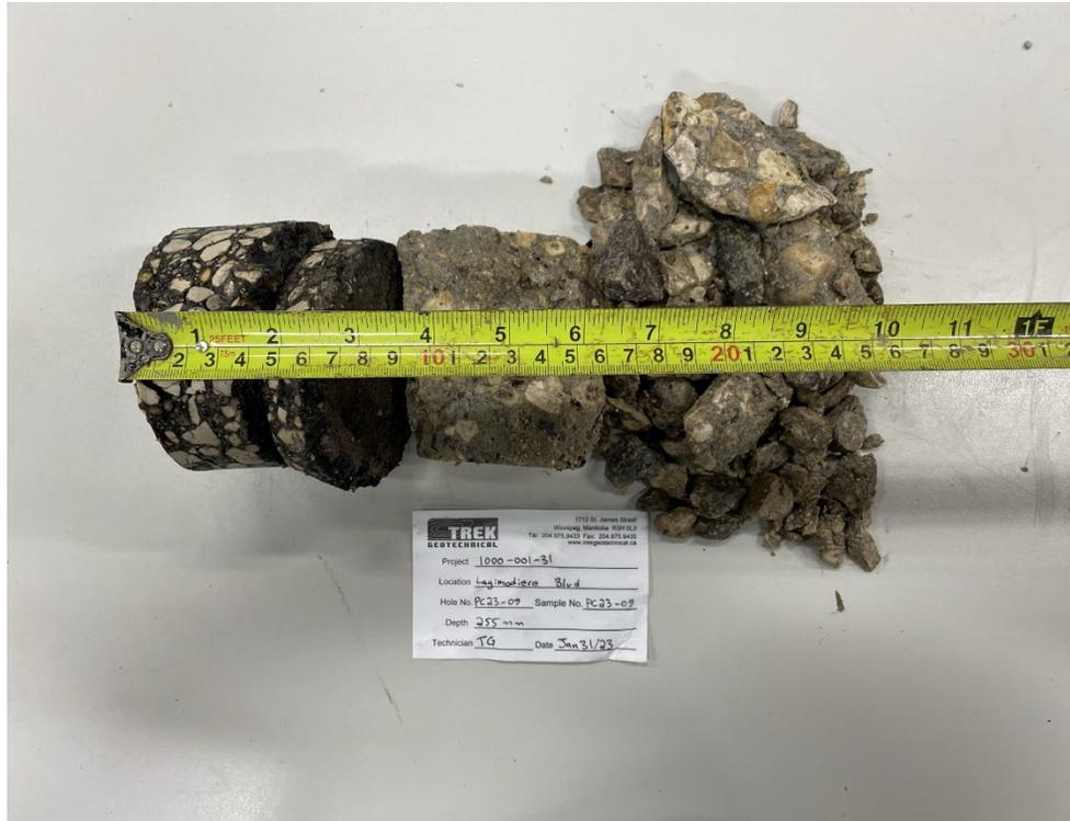
Photo 9: Pavement Core Sample PC-09
