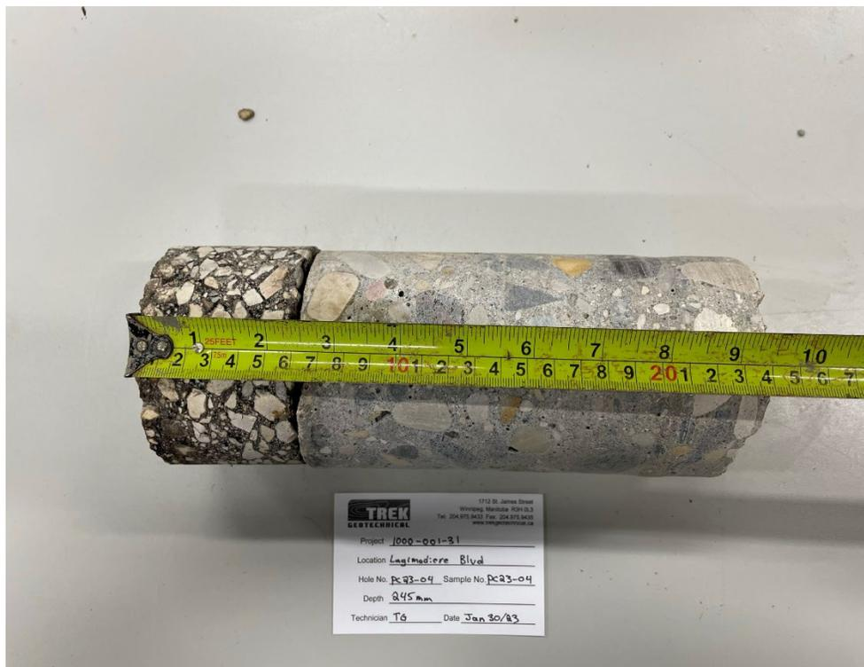
Photo 4: Pavement Core Sample PC-04
