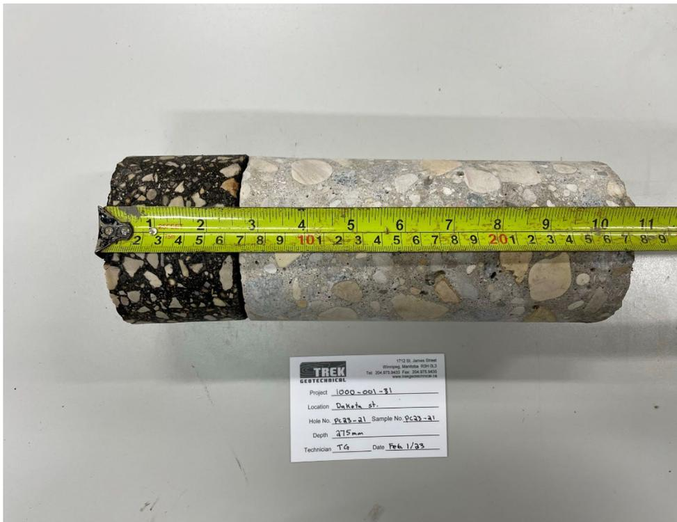
Photo 2: Pavement Core Sample PC-21
