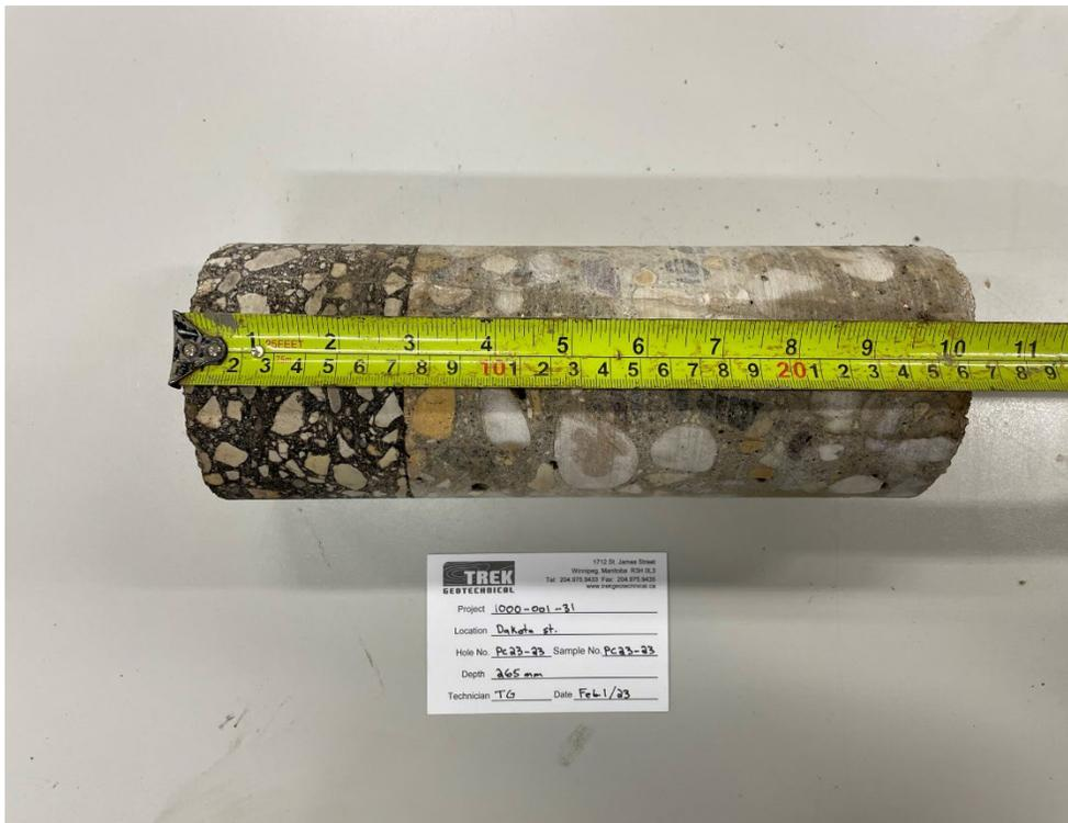
Photo 4: Pavement Core Sample PC-23
