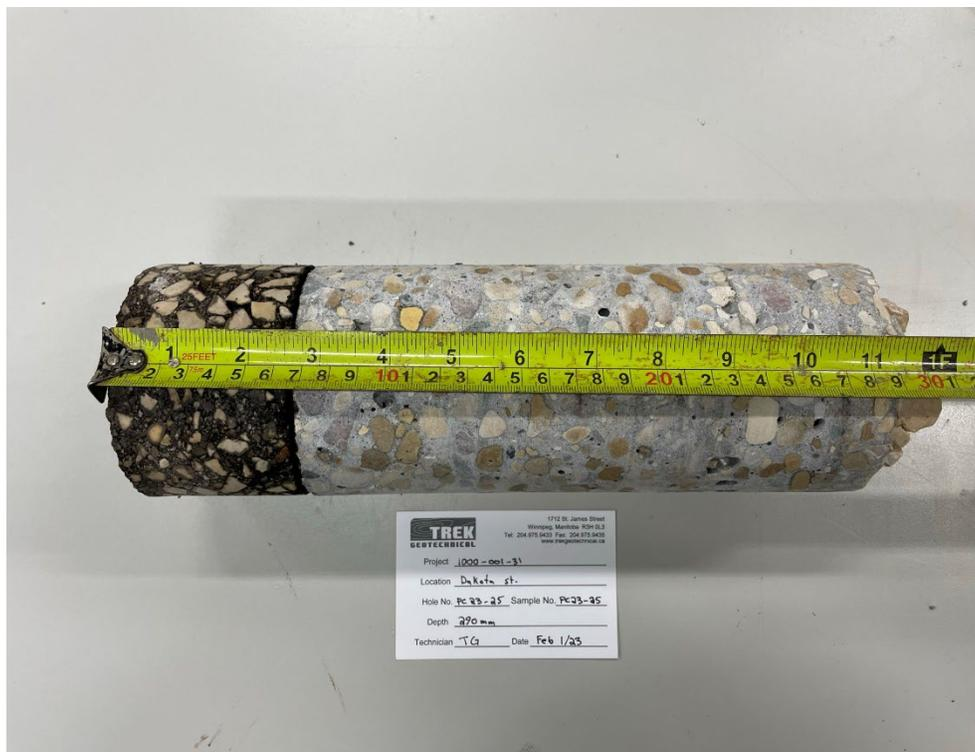
Photo 6: Pavement Core Sample PC-25
