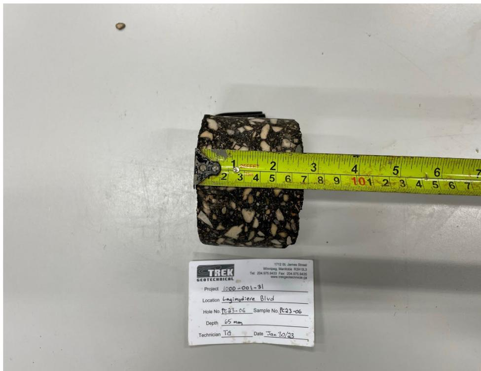
Photo 6: Pavement Core Sample PC-06
