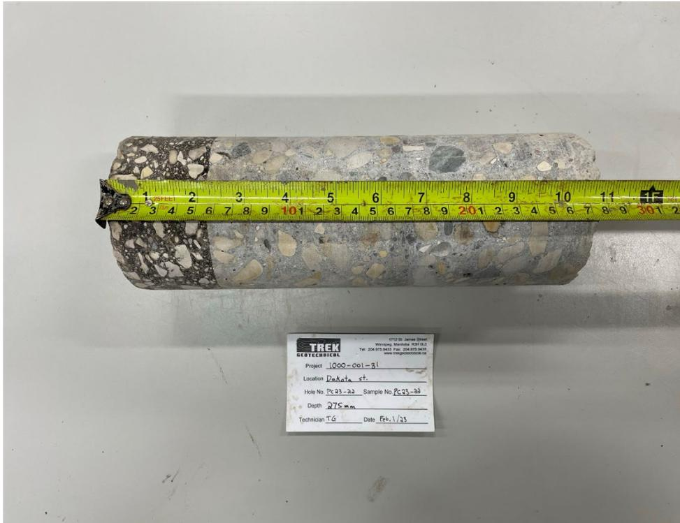
Photo 3: Pavement Core Sample PC-22
