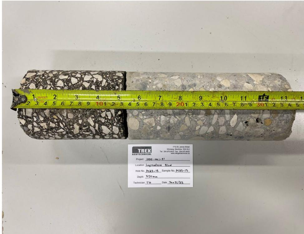
Photo 13: Pavement Core Sample PC-13
