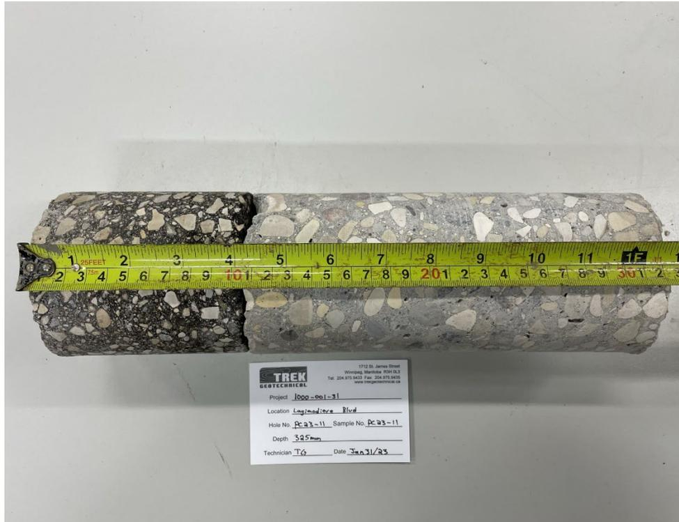
Photo 11: Pavement Core Sample PC-11
