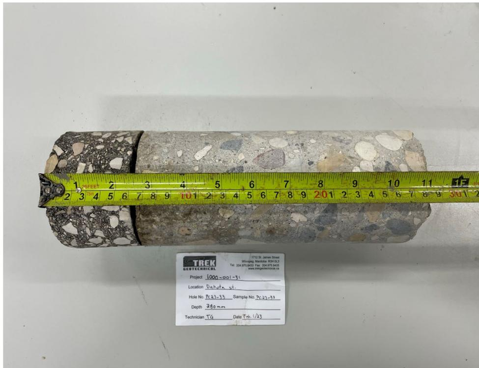
Photo 14: Pavement Core Sample PC-33
