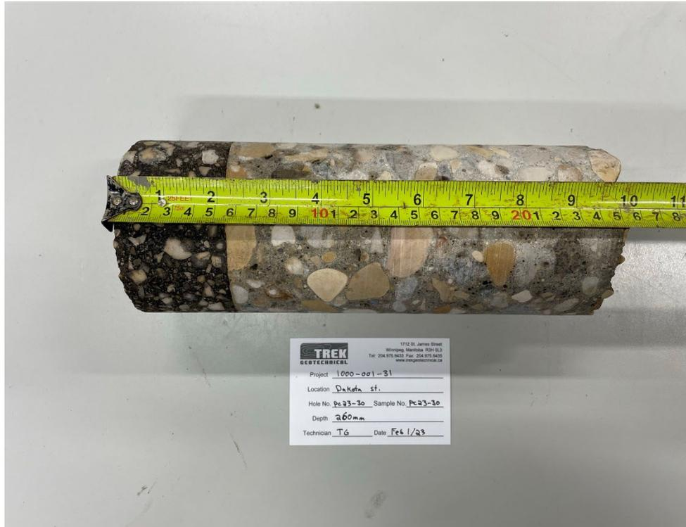
Photo 11: Pavement Core Sample PC-30
