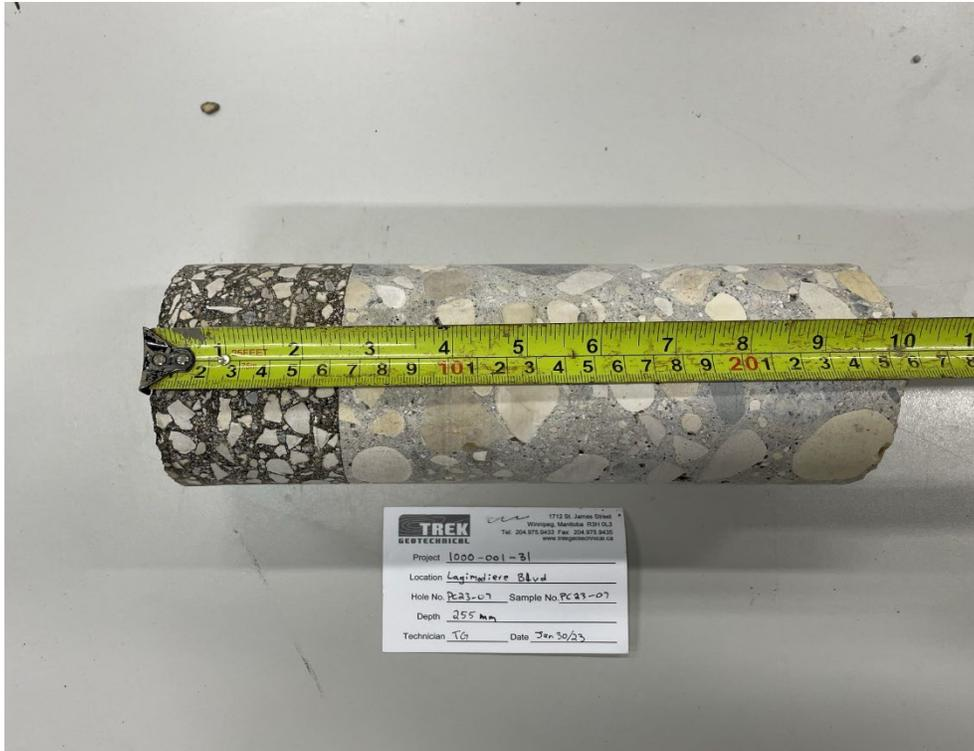
Photo 7: Pavement Core Sample PC-07
