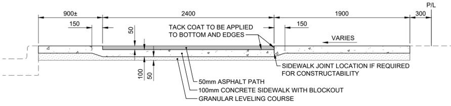
CONCRETE SIDEWALK WITH BLOCKOUT FOR ASPHALT PATH
