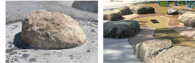
Ø750-1000mm BLACK GRANITE BOULDERS WITH FLAT / CUT FACE UNDERSIDE, ENSURE NO SHARP CORNERS, BOULDERS TO BE SELECTED AND APPROVED IN COORDINATION WITH CONTRACT ADMINISTRATOR
