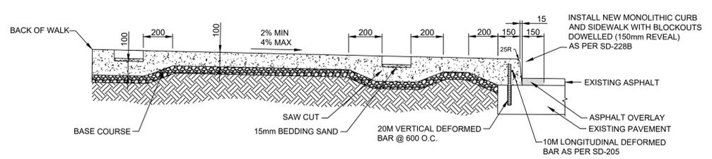
TYPICAL MONOLITHIC CURB AND SIDEWALK WITH BLOCKOUTS - SECTION VIEW
