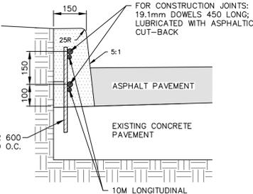
DETAIL 'A' - DOWELLED BARRIER CURB (SD-206A)
