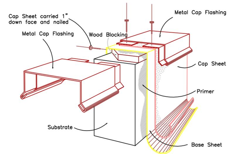
26 Gauge counter flashing complete with approx. 1/2" 45 degree bottom kick out is to be installed over all membrane stripping. Terminate flashing about 1" above top of new roofing. Do not install any fasteners behind the cap flashing and use only lap joints. This is to allow easy removal for future repairs.
