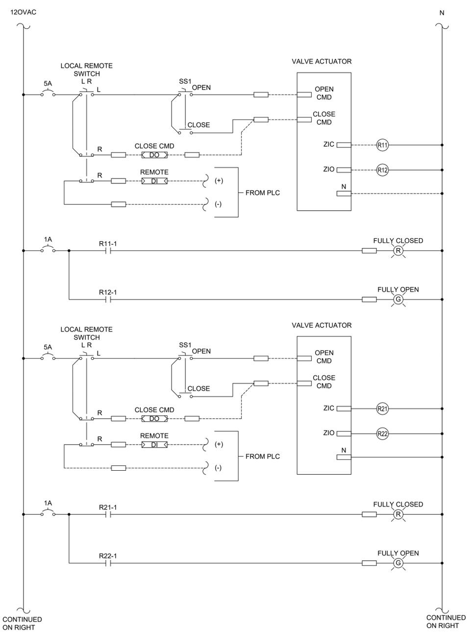
**1 | VALVE CONTROL STATION SCHEMATIC DIAGRAM (TYP)**
