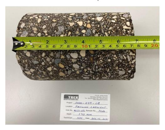
Photo 2: Pavement Core Sample at PC21-03
