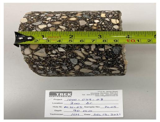
Photo 1: Pavement Core Sample at PC21-05
