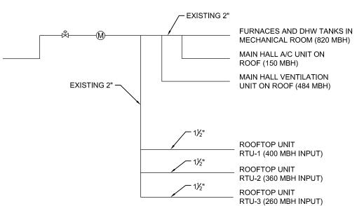
NATURAL GAS PIPING SCHEMATIC - EXISTING
