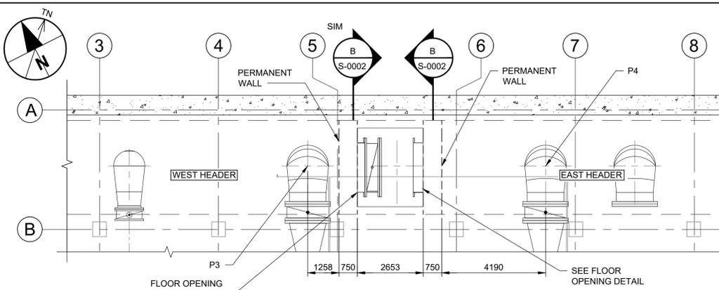
**STAGE 3 - EAST WALL, AND SPOOL, INSTALL - PLAN VIEW**
