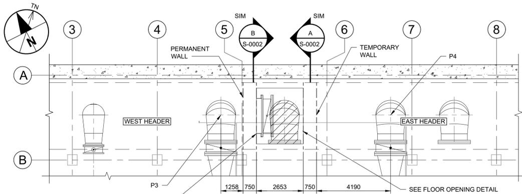
**STAGE 2 - WEST WALL, SPOOL, AND VALVE INSTALLATION - PLAN VIEW**
