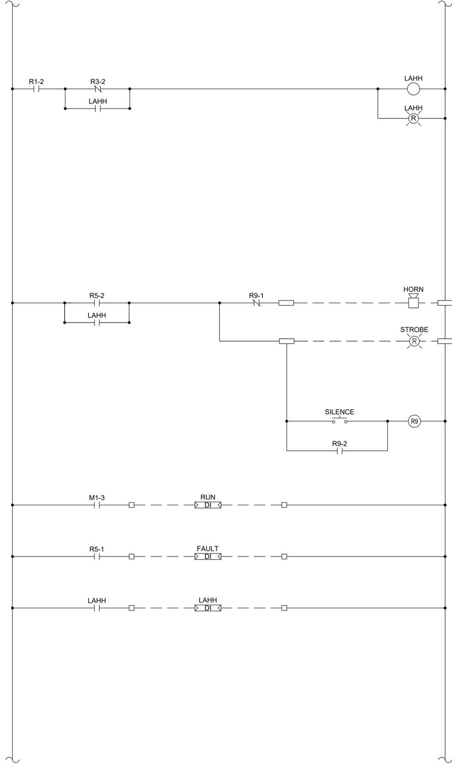
**1 SUMP PUMP SCHEMATIC DIAGRAM (TYP) CONTINUED**
