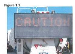
Figure 1.0 and 1.1: Tanker equipped with 4 beacons, retro-reflective striping and combined directional lighting/caution signage.
