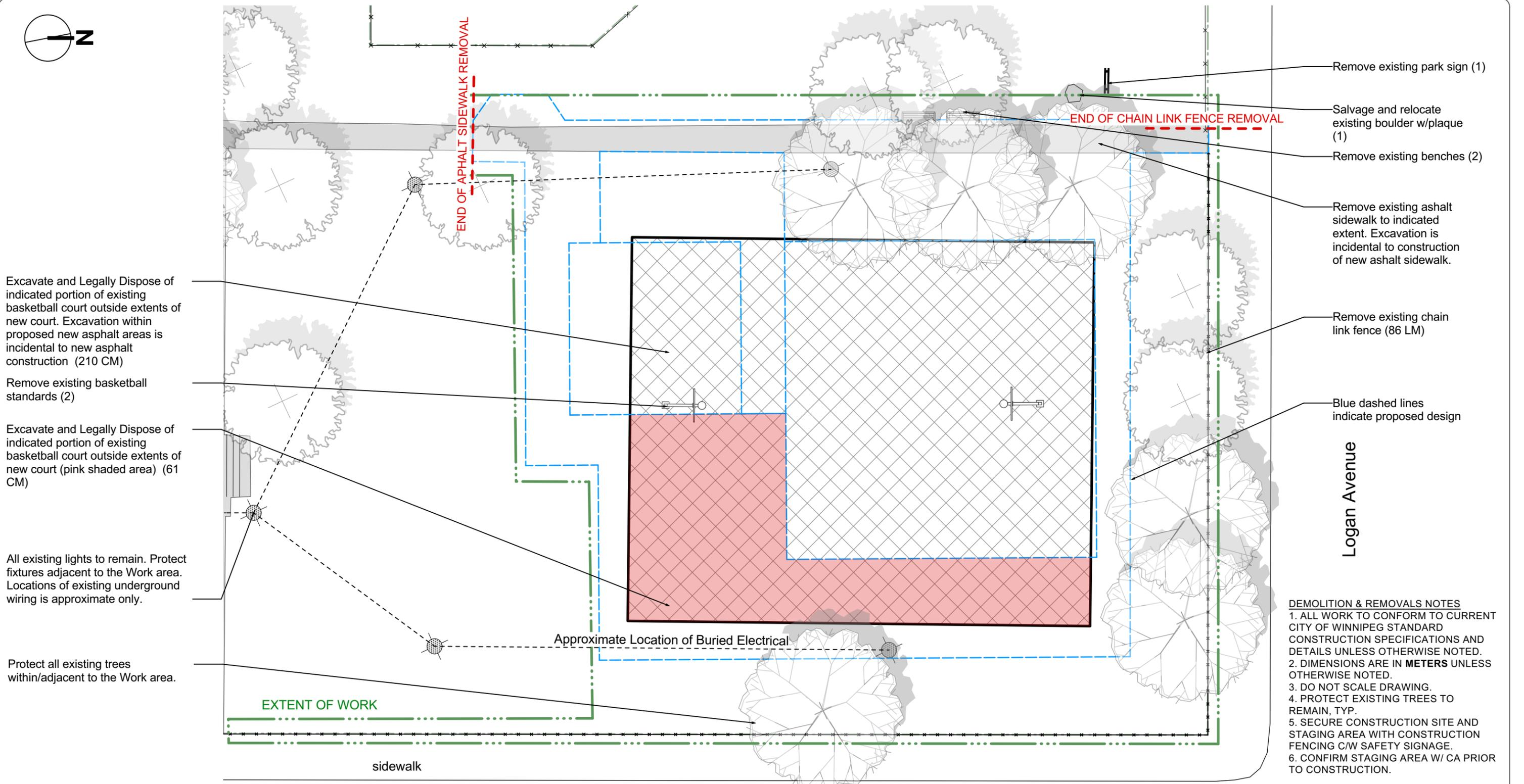
Excavate and Legally Dispose of indicated portion of existing basketball court outside extents of new court. Excavation within proposed new asphalt areas is incidental to new asphalt construction (210 CM)
