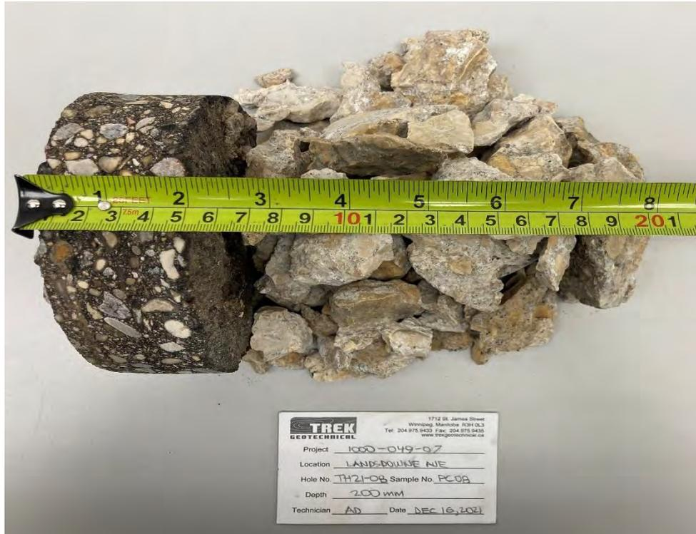
Photo 5: Pavement Core Sample at Test Hole TH21-08
