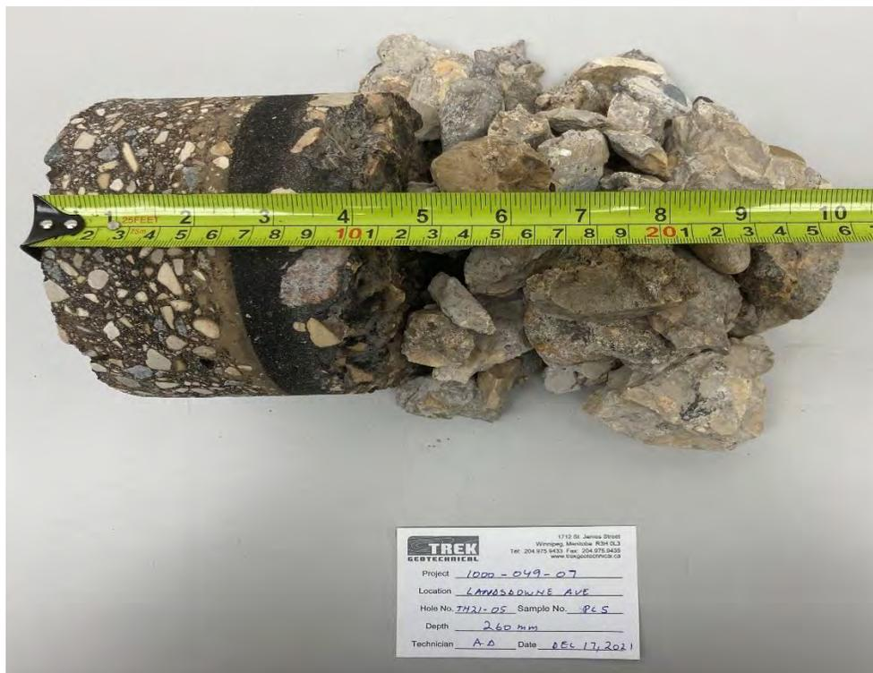
Photo 2: Pavement Core Sample at Test Hole TH21-05
