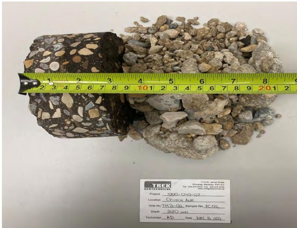
Photo 2: Pavement Core Sample at Test Hole TH21-02
