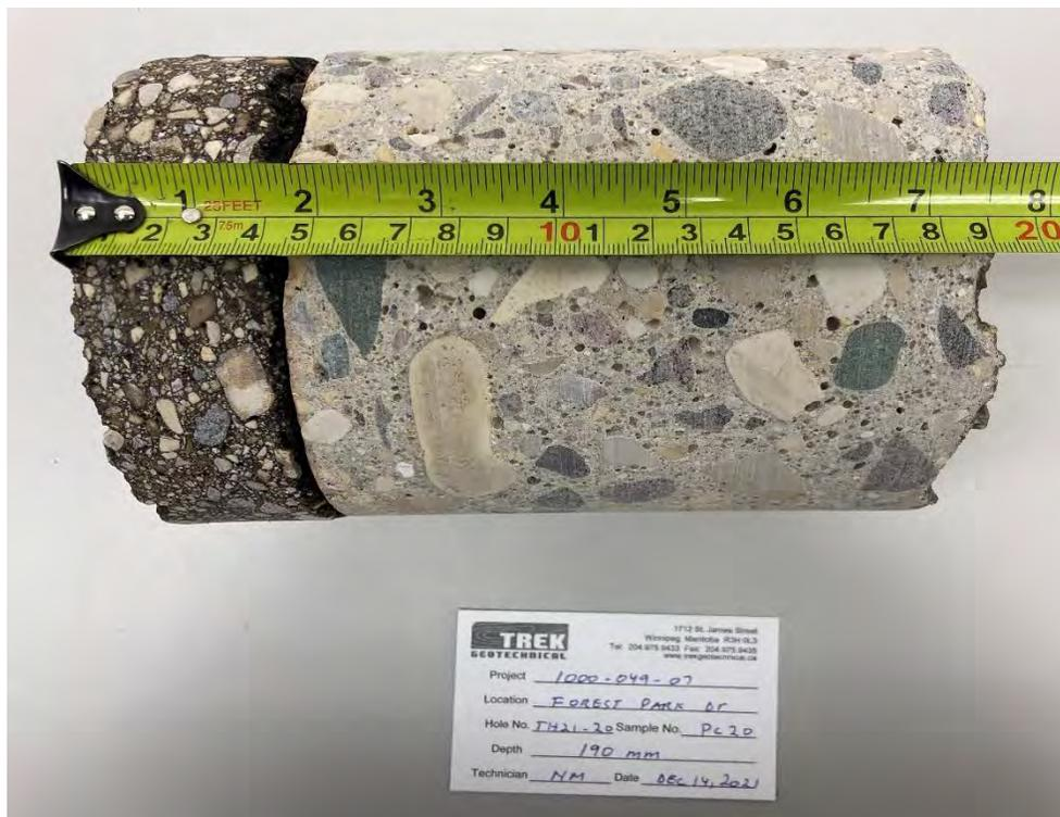
Photo 2: Pavement Core Sample at PC21-20
