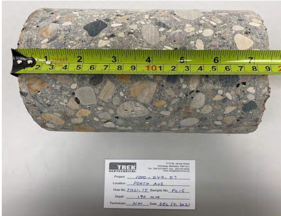
Photo 3: Pavement Core Sample at PC21-15
