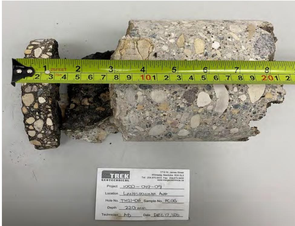
Photo 3: Pavement Core Sample at Test Hole TH21-06
