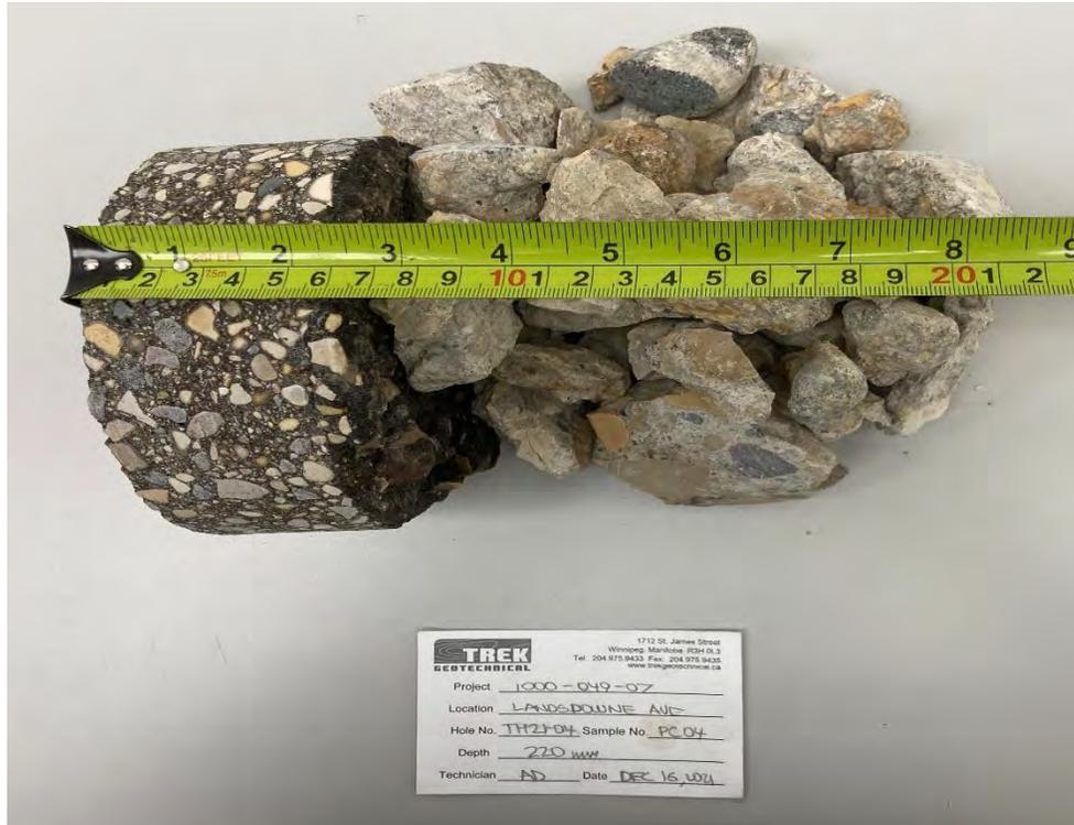
Photo 1: Pavement Core Sample at Test Hole TH21-04
