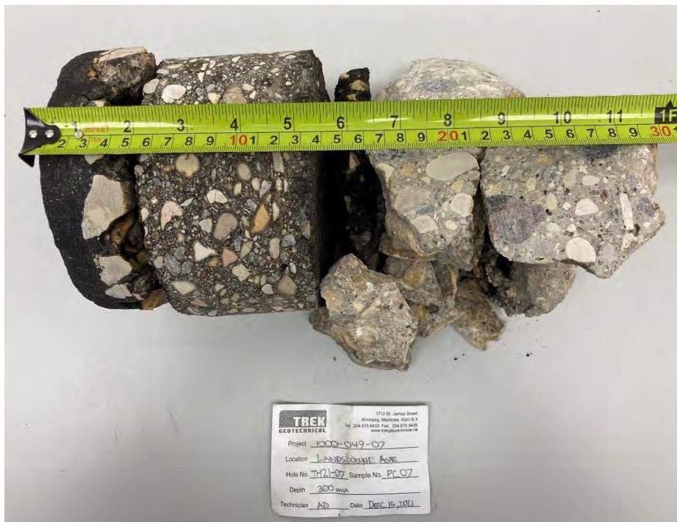
Photo 4: Pavement Core Sample at Test Hole TH21-07
