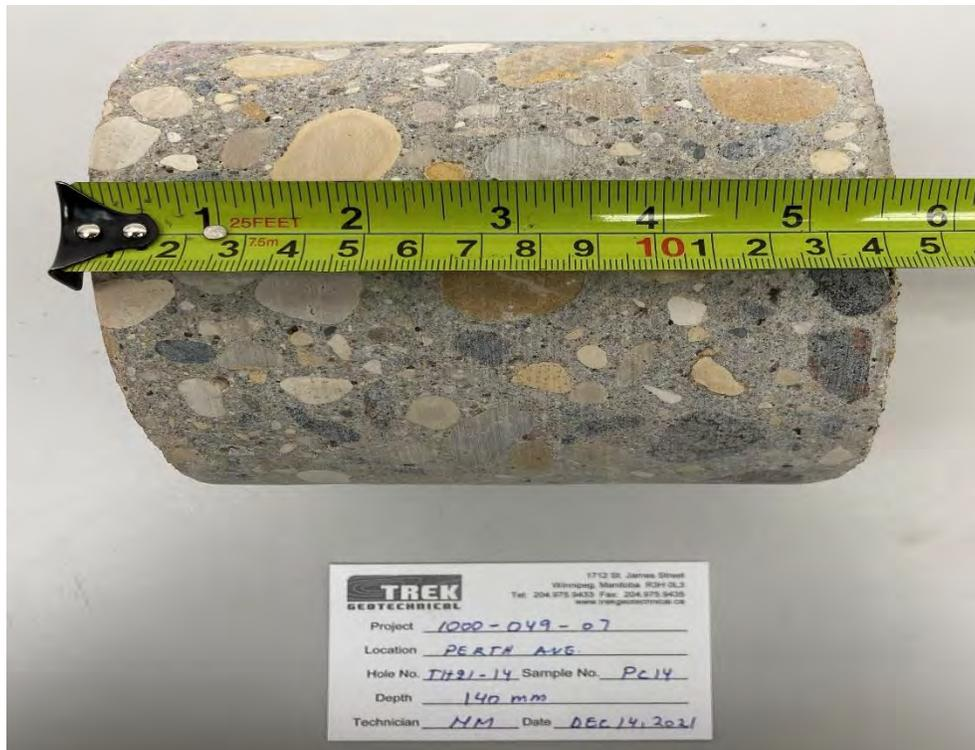
Photo 2: Pavement Core Sample at PC21-14
