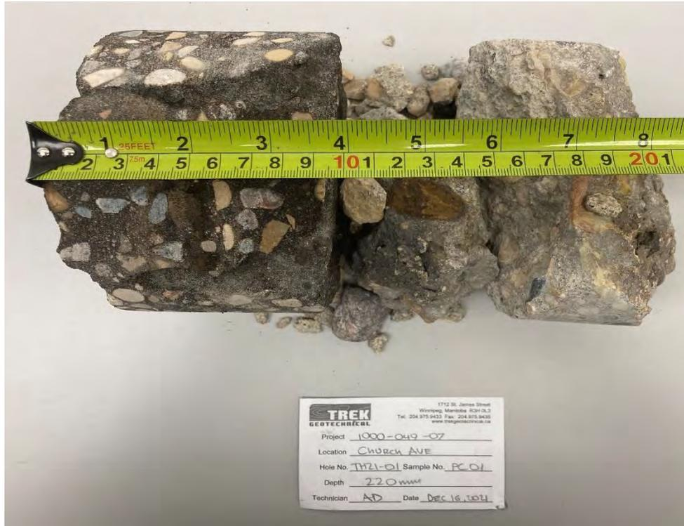
Photo 1: Pavement Core Sample at Test Hole TH21-01
