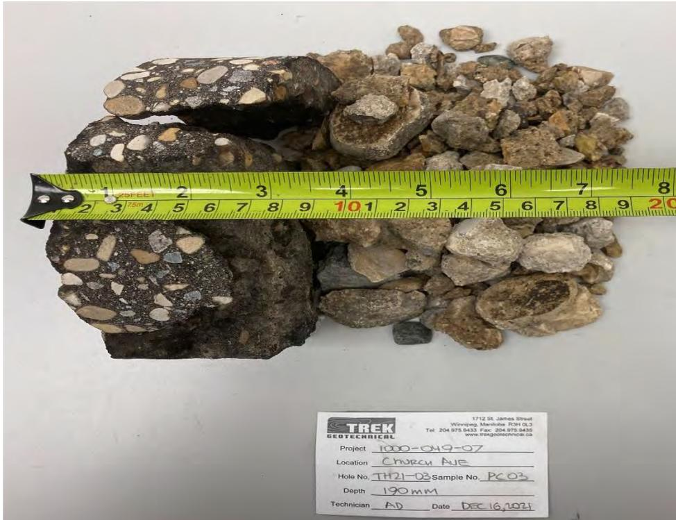
Photo 3: Pavement Core Sample at Test Hole TH21-03
