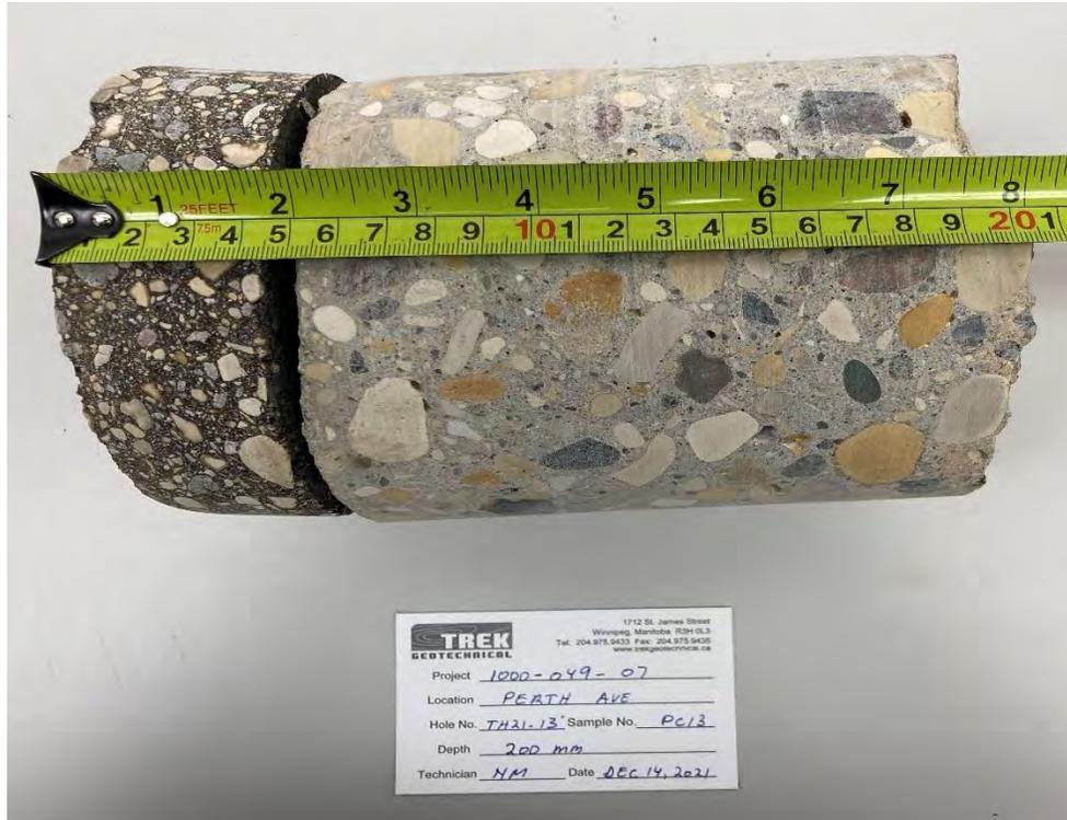
Photo 1: Pavement Core Sample at PC21-13
