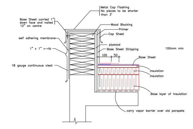
26 Gauge counter flashing complete with approx. 1/2" 45 degreee bottom kick out is to be installed over all membrane stripping. Terminate flashing about 1" above top of new roofing. Do not install any fasteners behind the cap flashing and use only lap joints. This is to allow easy removal for future repairs.
