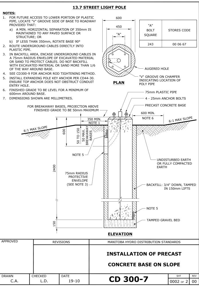
TO DEVELOP THE REQUIRED TENSION ON ANCHOR RODS, THE TURN-OF-NUT METHOD IS USED.
