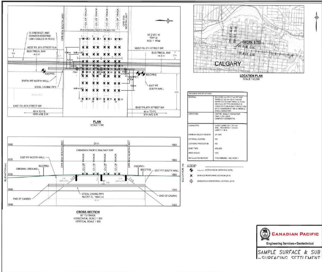
Figure A - Sample Surface and Subsurface Settlement Monitoring Layout
