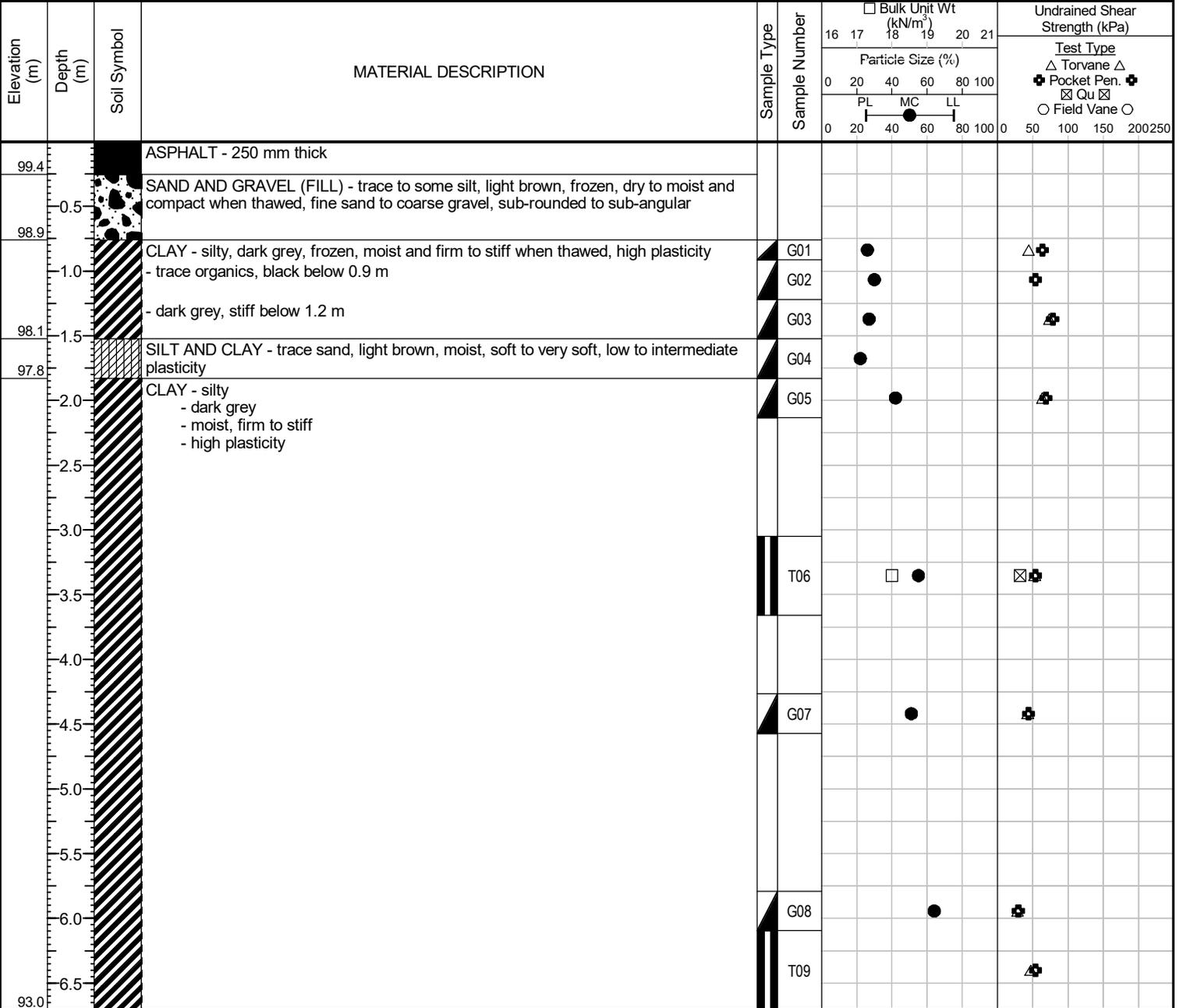
END OF TEST HOLE AT 6.9 m IN CLAY
