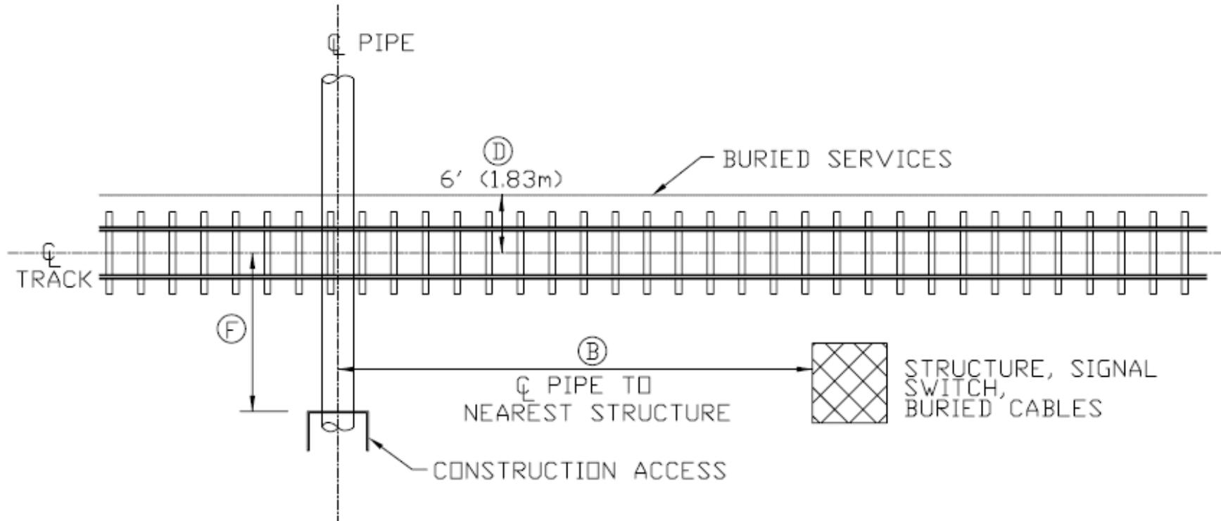
**Figure 1 – Plan of the proposed pipe crossing**
